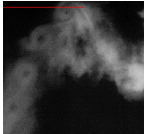
Fig. 2. Blade tip vortices from the 75%-test (rotor disk in red)
