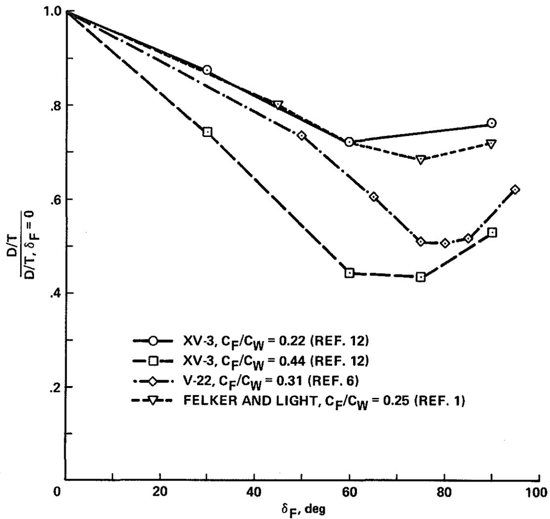
Figure 4. Effect of flap deflection on download. Data from small-scale wind tunnel tests.
