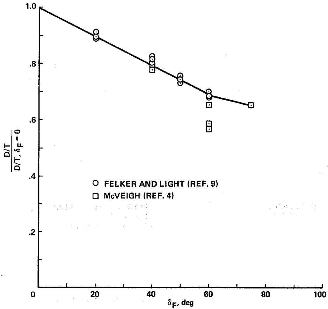
Figure 6. Effect of flap deflection of XV-15 aircraft download. Data from flight test.
