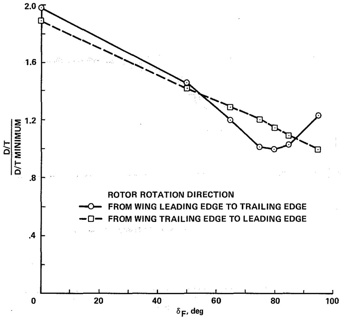
Figure 11. Effect of rotor rotation direction on download. Data from Ref. 6. Minimum download was equal in both cases.
