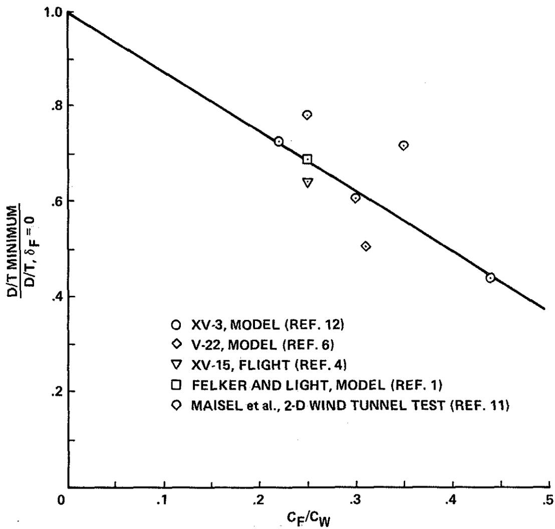
Figure 5. Effect of flap size on maximum flap download reduction.
