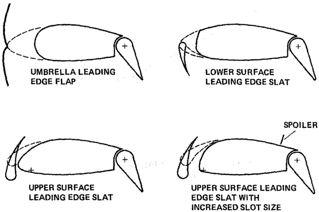
Figure 7. Typical leading-edge devices for download reduction (Ref. 11).
