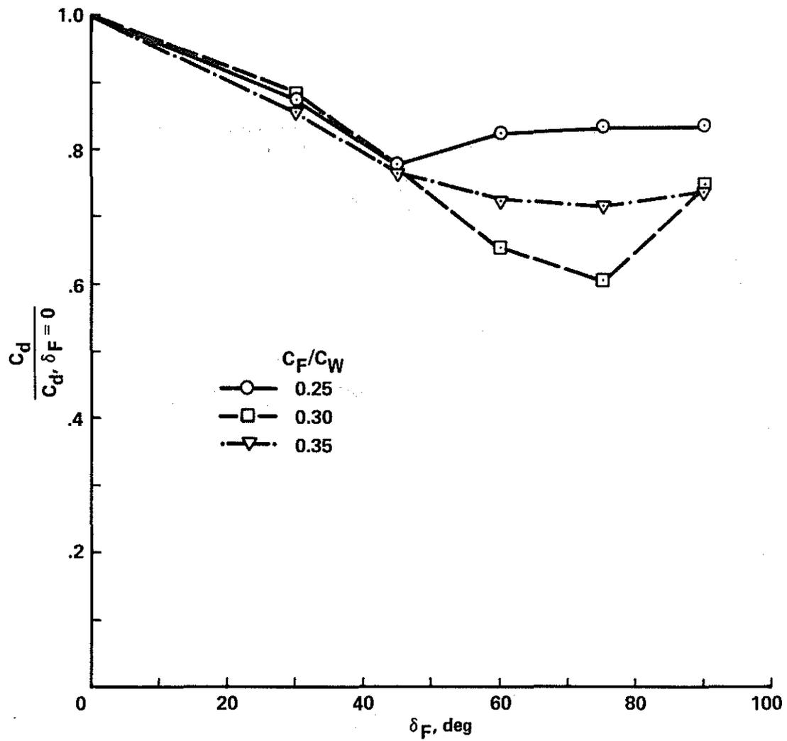
Figure 3. Effect of flap deflection on drag of various flapped airfoils at  $-90^\circ$  angle of attack. Data from 2-dimensional wind tunnel test (Ref. 11).
