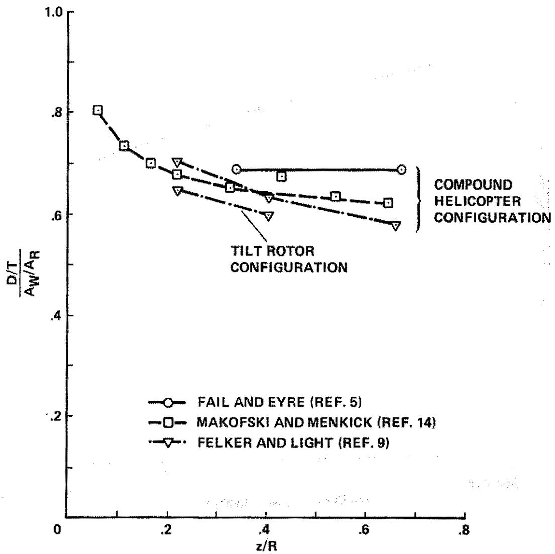
Figure 8. Effect of distance between rotor and wing on download.
