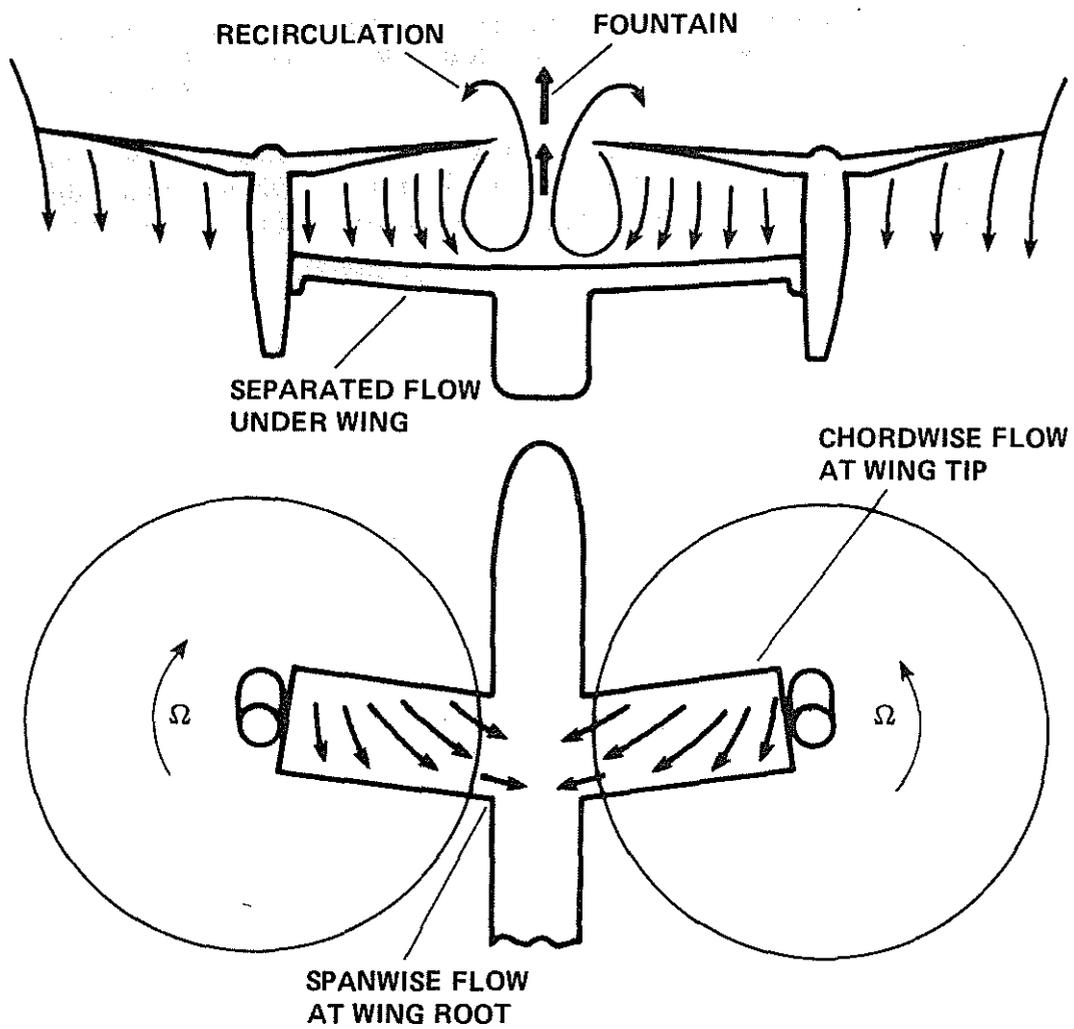
Figure 1. Schematic of rotor/wing flow field.
