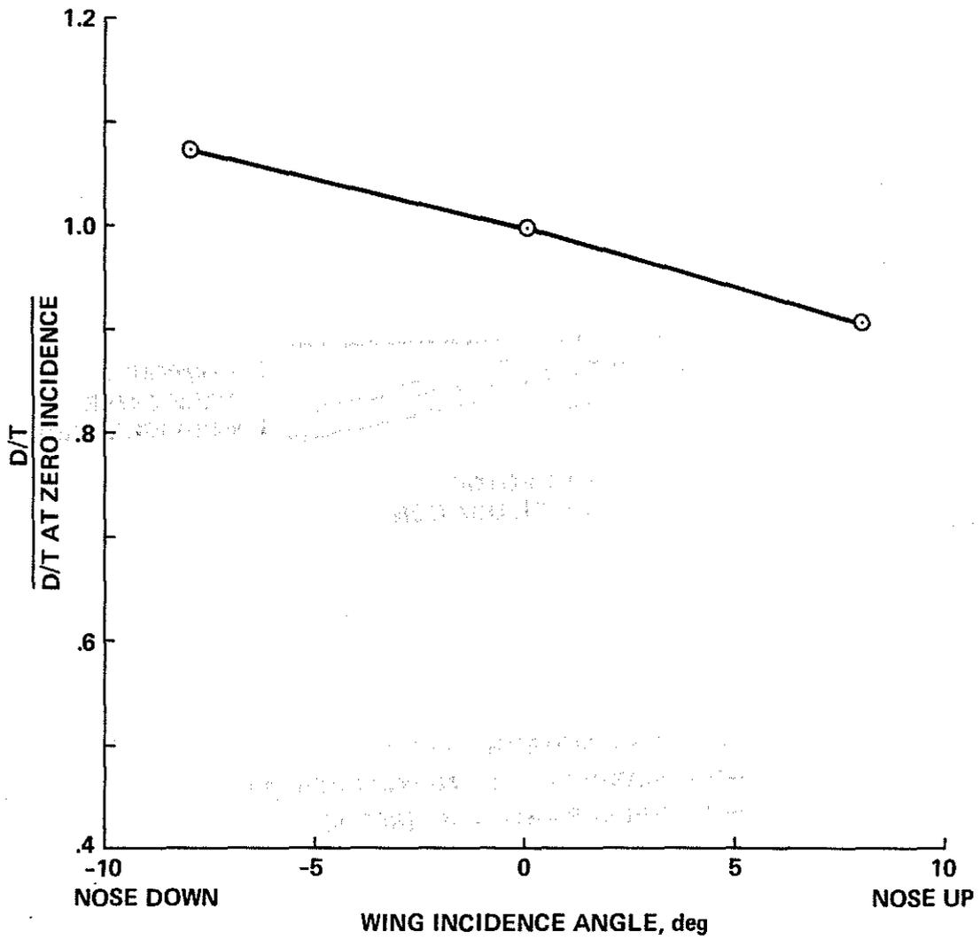
Figure 9. Effect of wing incidence angle on download. 60° flap deflection. Data from Ref. 1.
