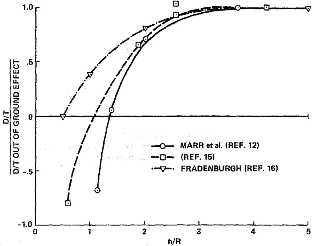
Figure 10. Effect of distance between rotor and ground on download.
