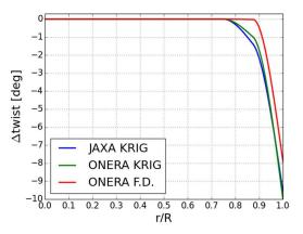
Fig. 7. Results of optimal twist distribution at blade tip portion in hovering. [5]
