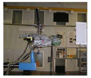
Fig. 3. HOTIS (HOver TIp vortex Structure test) setup. [10]
