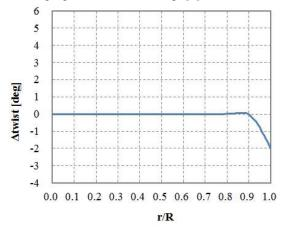
Fig. 9. Result of optimal twist distribution at blade tip portion in forward flight.
