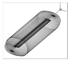
Fig. 6. JAXA CFD grid around blade.
