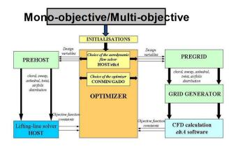
Fig. 1. ONERA existing CFD based rotor optimization framework.
