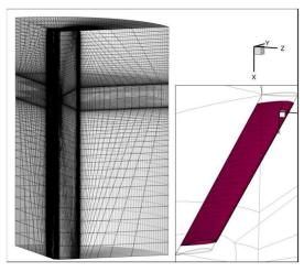
Fig. 5. ONERA CFD grid around blade.
