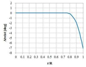
Fig. 12. Result of multi-point optimal twist distribution at blade tip portion.
