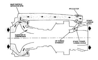
The RTM322 engine incorporates a unique Inlet Particle Separator (IPS) module. This unit, having no moving components, utilises an inter – stage turbine ejector bleed system in combination with vortex separation of airborne particles via the ballistic/aerodynamic design of the IPS scroll. Testing to MIL-E-50007 requirements has demonstrated particle separation efficiencies in the mid 90% range.
