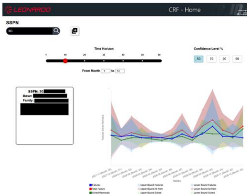
Figure 2: Component Removal Forecast user interface. The forecast of the need of a component at Part Number level is presented considering the prediction of both scheduled (e.g., overhaul time or retirement life) or un-scheduled (e.g., malfunction or failure) events represented adopting different colours. The name and technical detail of the PN component have been blurred.
