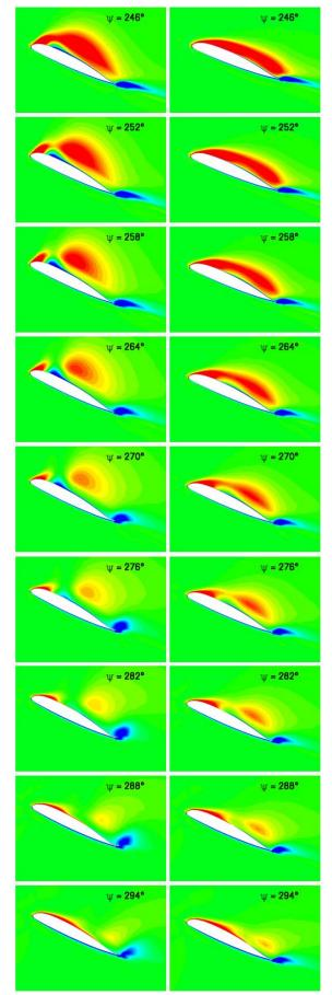
Figure 18: Timewise evolution of spanwise vorticity, r/R = 0.5 (left: passive, right: rigid flap)
