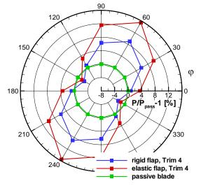
Figure 8: Rotor power over phase angle, trim 4
