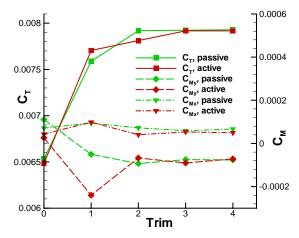
Figure 24: Mean values of rotor load coefficients versus trim iteration
