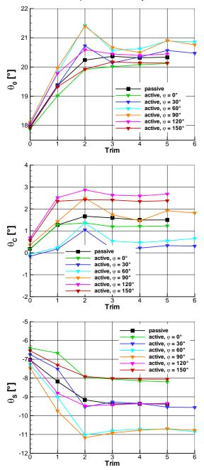
Figure 23: Convergence of collective and cyclic pitch angles
