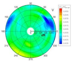
Figure 15:  $\Delta C_{Fy}Ma^2$ -distribution, elastic trailing edge rotor minus rigid flap rotor
