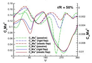
Figure 11: Comparison of azimuthal load distributions (r/R = 0.50)
