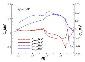
Figure 25: Comparison between HOST loads and CFD loads in trimmed state,  $\psi$ =60°
