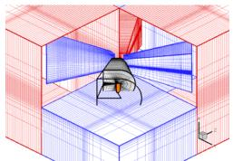
Figure 1: Chimera grid setup
