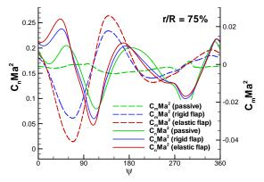
Figure 10: Comparison of azimuthal load distributions (r/R = 0.75)
