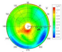
Figure 12:  $C_{Fv}Ma^2$ -distribution, passive rotor
