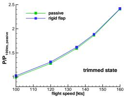
Figure 20: Relative power consumption, reference power: passive rotor at 100kts
