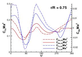
Figure 26: Comparison between HOST loads and CFD loads in trimmed state, r/R = 0.75
