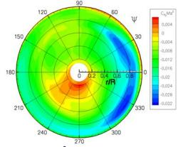
Figure 13:  $C_{Fy}Ma^2$ -distribution, rigid flap rotor
