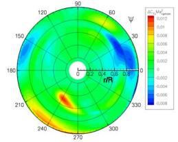
Figure 14:  $\Delta C_{Fy}Ma^2$ -distribution, rigid flap rotor minus passive rotor
