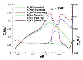
Figure 9: Comparison of radial load distributions
