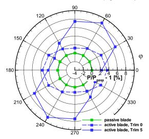
Figure 27: Rotor power over phase angle
