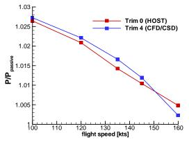
Figure 21: Relative power consumption, reference power: passive rotor at same speed
