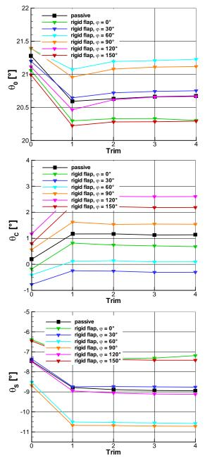
Figure 4: Convergence of collective and cyclic pitch angles
