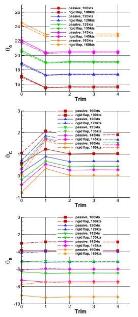
Figure 19: Convergence of collective and cyclic pitch angles
