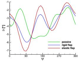
Figure 17: Comparison of elastic blade tip torsion
