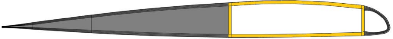
Figure 5. Idealized UH-60A blade cross section with highlighted spar
