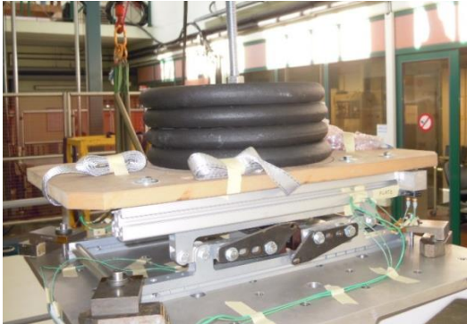
Figure 3: First prototype of seat sarib with mass on shaker
