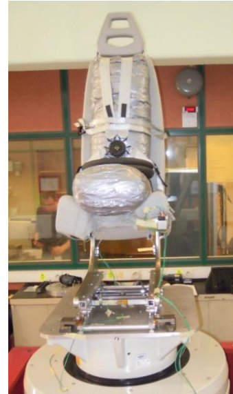
Figure 5: First prototype of seat sarib with Fisher H160 seat and ballasts
