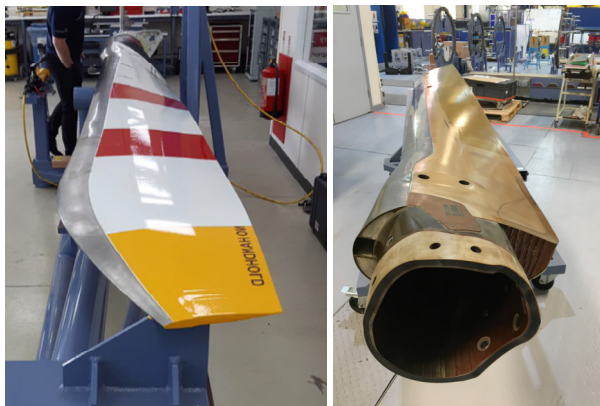
Figure 18 –New generation Enhanced Tiltrotor Blade (NGCTR-TD aircraft, Ref. 6)
