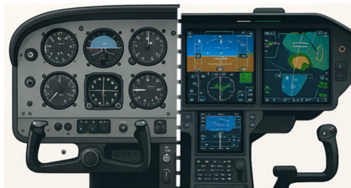
Figure 24 - Comparison between past (WE-01, left) and modern cockpits (AW609, right)
