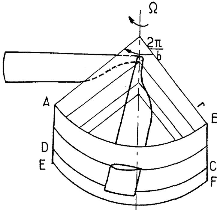
The contribution of branch DA to circulation will be balanced by the circulation along BC. The circulation along the contour ABCD defined in the figure above is then reduced to circulation along AB and CD. Moreover, it can be noticed that the variation with  $\Psi$  of the  $U$  component in any point of AB
