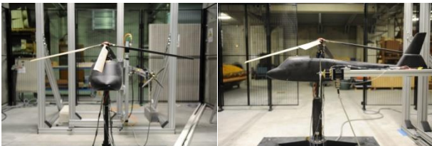
Figure 2: ONERA test rig for Rotor / Propeller wake interaction study
