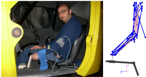
Figure 4. Test subject inside the flight simulator grasping the collective lever (left) and multibody model of the pilot's arm (right).
