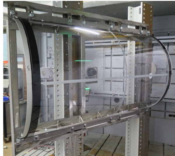
Figure 3: Experimental setup without speckle film
