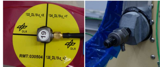
Figure 5: Sticker to mark positions for accelerometers on helicopter (left), 3D-printed adapter to introduce forces (right)
