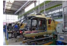
H/C a | Station IV: Assembly (LG+CFS+BS)
