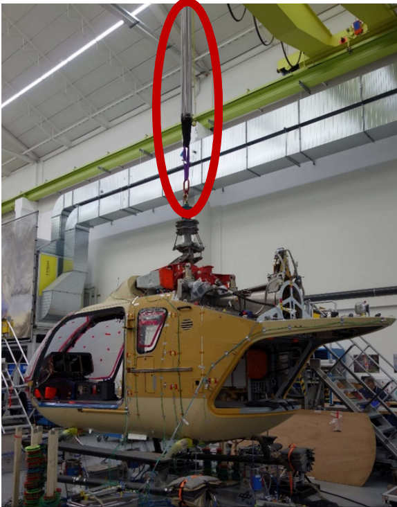
Figure 4: Helicopter softly suspended using bungee cords from the hall crane (highlighted in red)
