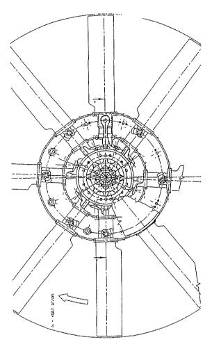
The mechanical systems feature the minimum number of parts and high-performance, well-ageing materials: dural casings; latest-design, surface-hardened teeth, stainless steel rotor mast, new grade, little notch-effect sensitive titanium rotor hub, MMC (dural with silica inclusions).
