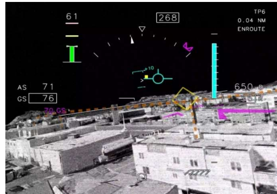
Figure 8. The Primary Flight Display (PFD) Integrated Cueing Environment-Collision Avoidance Symbology (ICE-CAS) overlaid on the Forward Looking InfraRed (FLIR) image. In this Figure, the yellow diamond indicates the most urgent obstacle. The Diamond's color indicates the threat level from 0 (yellow) to 1 (red). A conformal line is superimposed over powerline wires and towers with the color indicating clearance, orange below, blue cleared.
