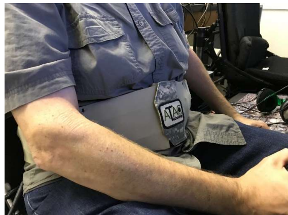
Figure 16. The Tactile Situational Awareness System (TSAS). The belt provides obstacle cueing from 12 directions, 0° forward to 330° in 30° increments.
