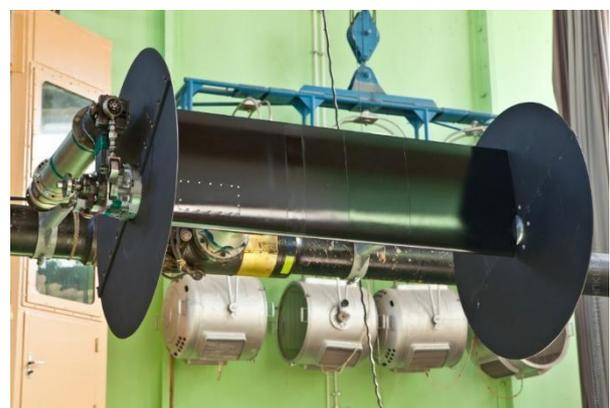
Figure 2: General view of the wing model on the “Dynamic Wing” rig.
