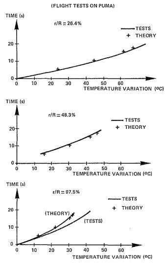
Fig. 14 : TEMPERATURES AT DEICING MAT/BLADE INTERFACE
