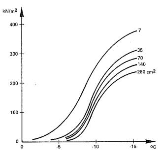
Fig. 19 : SHEDDING STRESS VALUES ACCORDING TO TEMPERATURE AND TO ICED AREA
