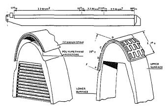
Fig. 3 : SA 330 AND AS 332 DEICED MAIN ROTOR BLADE
