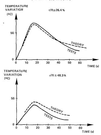
Fig. 15 : TEMPERATURES AT DEICING MAT/ BLADE INTERFACE
