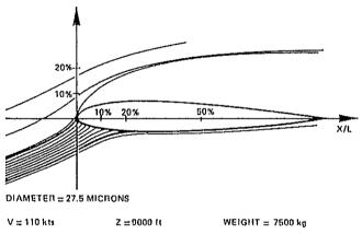
Fig. 10 : DROPLET TRAJECTORIES CALCULATION
