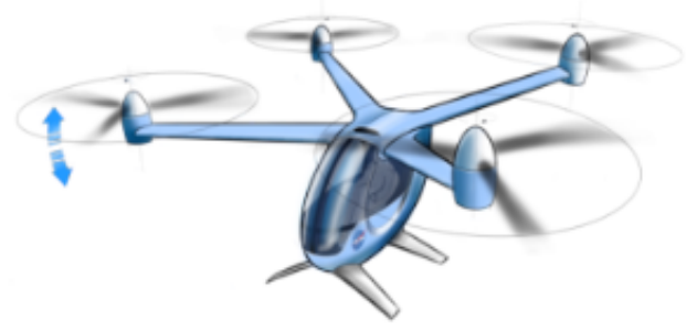
Figure 1. Layout of the one-passenger NASA CRM electric quad-rotor configuration (Ref. 10).
