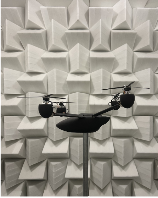
Figure 5. Quad-rotor model set up in the anechoic test chamber.
