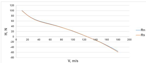
Fig. 17. Longitudinal force, perpendicular to the shaft axis, normal rotor ( $R_n$ ) and stiffened rotor ( $R_s$ )
