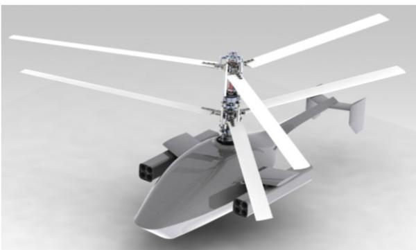
Fig. 4. Coaxial rotor implemented in a concept hull
