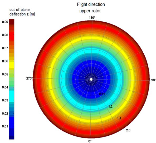
Fig. 6. Distribution of out-of-plane blade deflection at rotor disks in hover with for upper rotor
