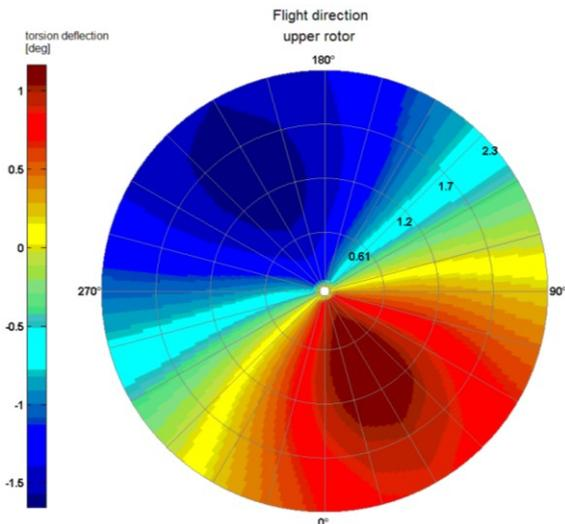
Fig. 22. Distribution of torsion blade deflection at disk of upper rotor, in level flight at speed of  $V=100$  km/h (for stiffened rotor  $R_s$ )
