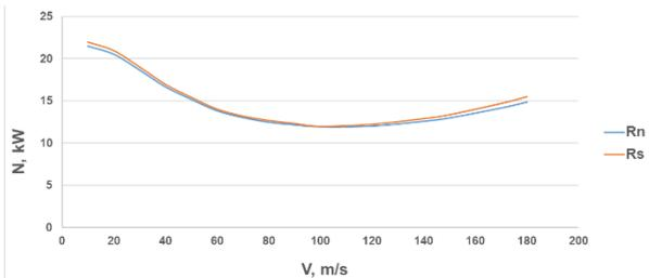
Fig. 16. Power consumption of normal rotor ( $R_n$ ) and stiffened rotor ( $R_s$ )
