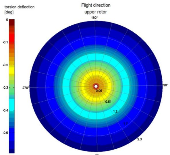
Fig. 8. Distribution of torsion blade deflection at rotor disks in hover with for upper rotor
