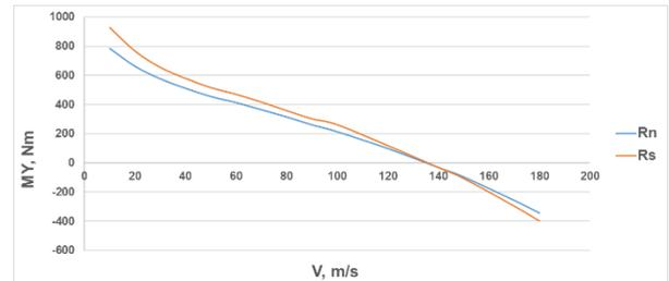
Fig. 20. Pitching moment (diving), for normal rotor ( $R_n$ ) and stiffened rotor ( $R_s$ )
