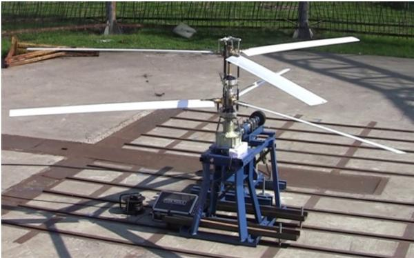
Fig. 2. Coaxial rotor on a test stand
