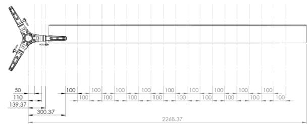
Fig. 5. Rotor hub arms and rotor blade cross-section
