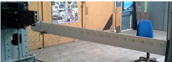
Fig. 3. Coaxial rotor blade stiffness measurement
