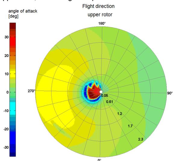
Fig. 14. Distribution of local angle of attack for disk of upper rotor in level flight at speed of  $V=100$  km/h
