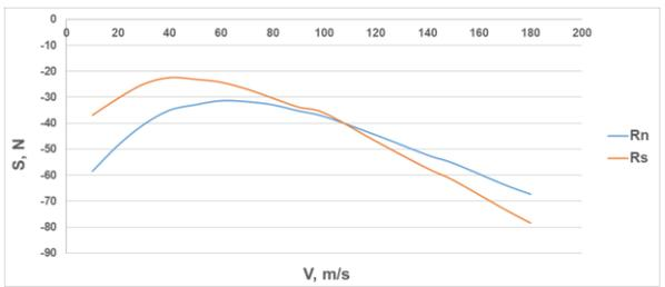
Fig. 18. Lateral force, perpendicular to the shaft axis, (azimuth  $90^\circ$ ), normal rotor ( $R_n$ ) and stiffened rotor ( $R_s$ )
