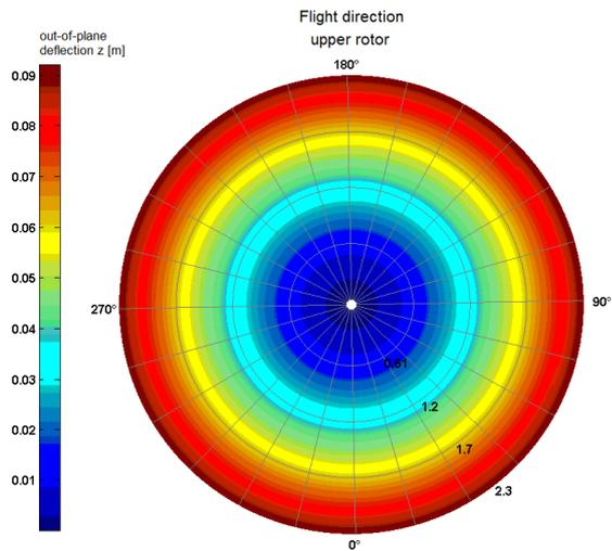
Fig. 10. Distribution of out-of-plane blade deflection at rotor disks in hover with vertical velocity of 2.5 m/s for lower rotor
