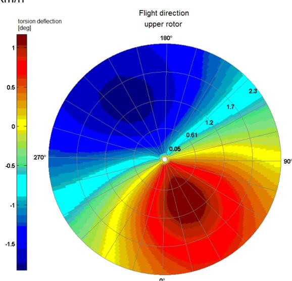
Fig. 13. Distribution of torsion blade deflection at disk of upper rotor, in level flight at speed of  $V=100$  km/h
