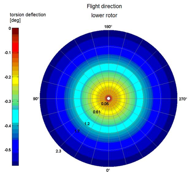
Fig. 9. Distribution of torsion blade deflection at rotor disks in hover with for lower rotor
