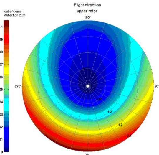
Fig. 12. Distribution of out-of-plane blade deflection at disk of upper rotor, in level flight at speed of  $V=100$  km/h
