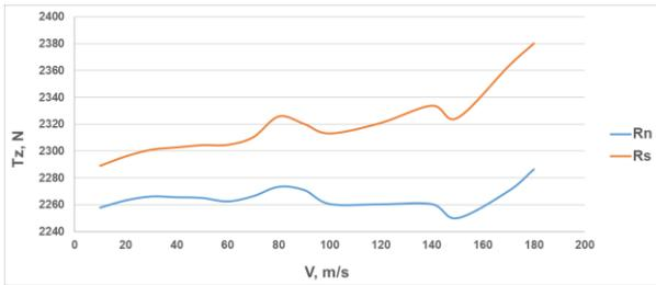
Fig. 15. Thrust, for normal rotor ( $R_n$ ) and stiffened rotor ( $R_s$ )
