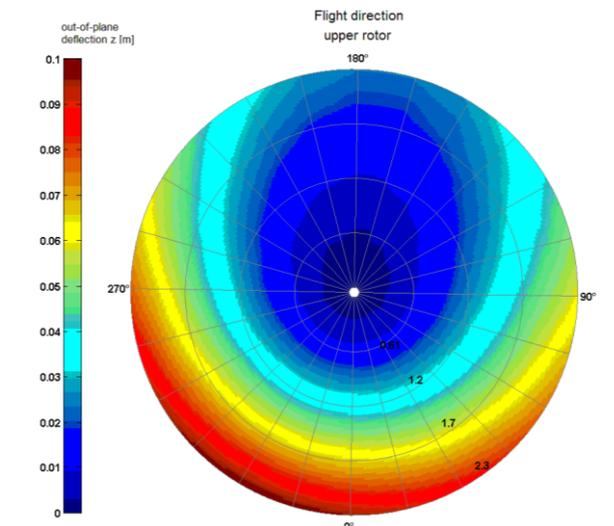
Fig. 21. Distribution of out-of-plane blade deflection at disk of upper rotor, in level flight at speed of  $V=100$  km/h (for stified rotor  $R_s$ )
