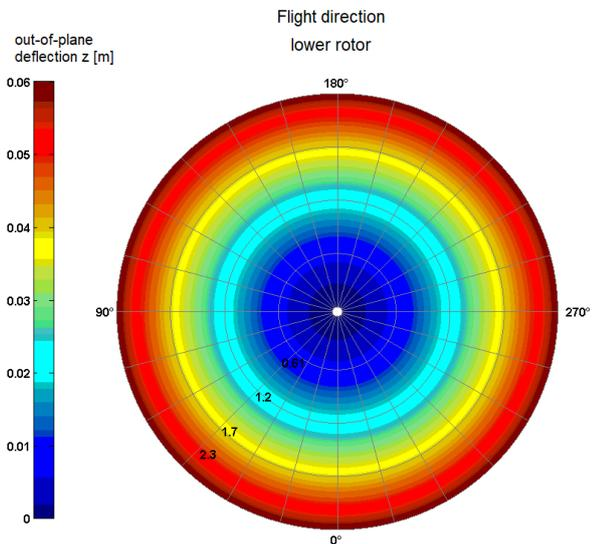
Fig. 7. Distribution of out-of-plane blade deflection at rotor disks in hover with for lower rotor
