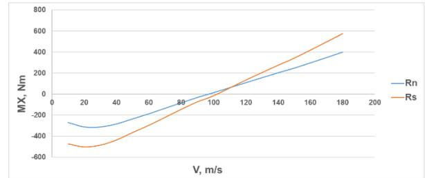
Fig. 19. Rolling moment (azimuth  $270^\circ$ ), for normal rotor ( $R_n$ ) and stiffened rotor ( $R_s$ )
