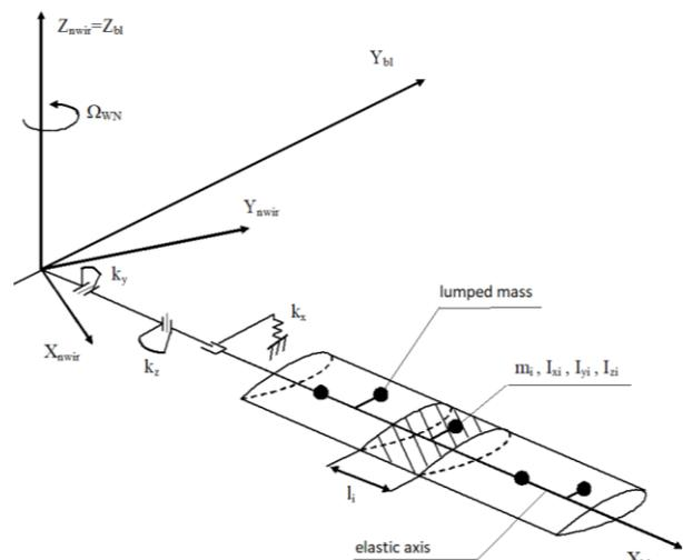
Fig. 1. Physical model of helicopter rotor includes blade elastic axes with sets of lumped masses [8]
