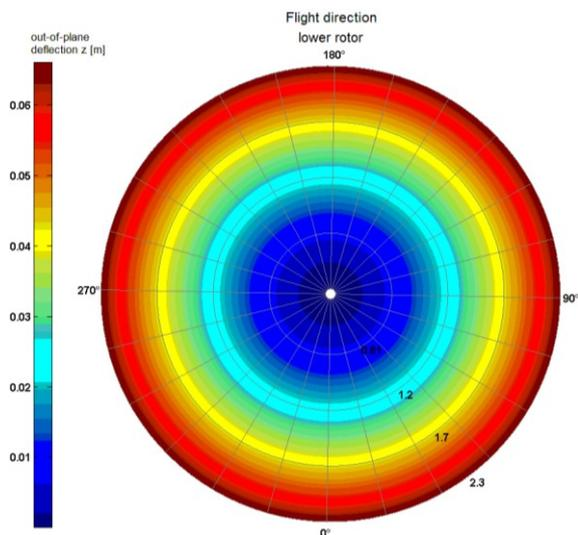
Fig. 11. Distribution of out-of-plane blade deflection at rotor disks in hover with vertical velocity of 2.5 m/s for lower rotor
