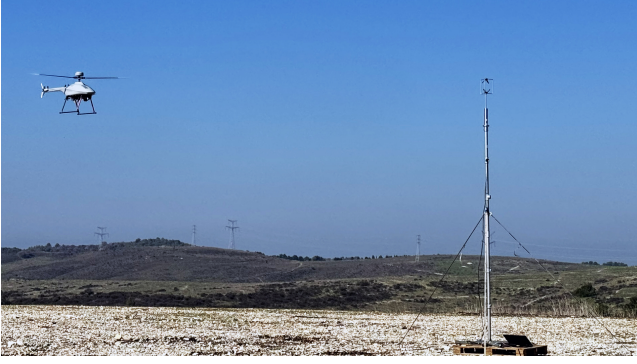
Figure 2. Flight test with a wind sensor
