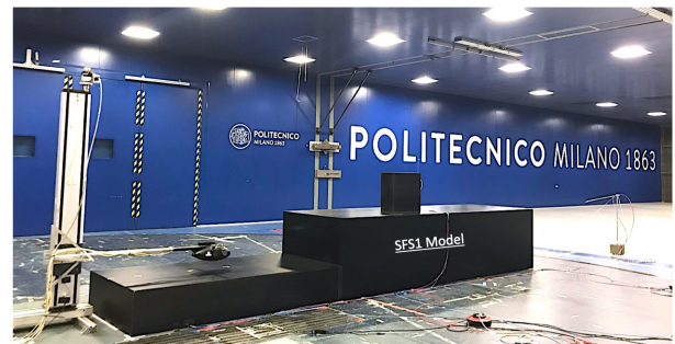
Figure 1: The test rig mounted inside the GVPM.
