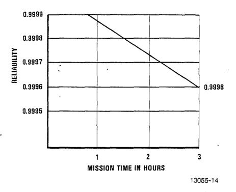
Figure 13. System Reliability as a Function of Time
