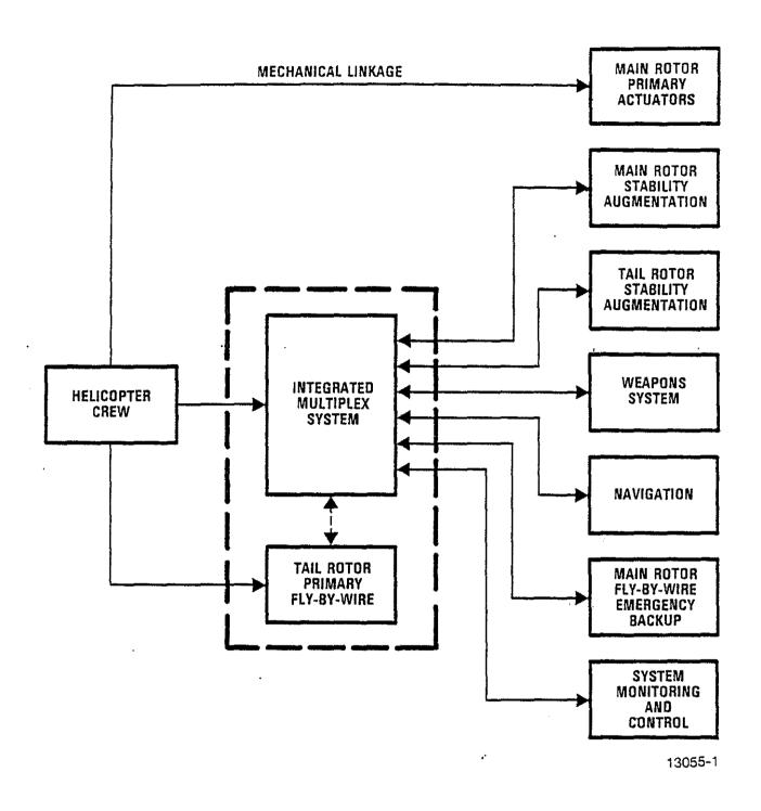
Figure 1. Primary Functions of the Integrated Multiplex Syst
