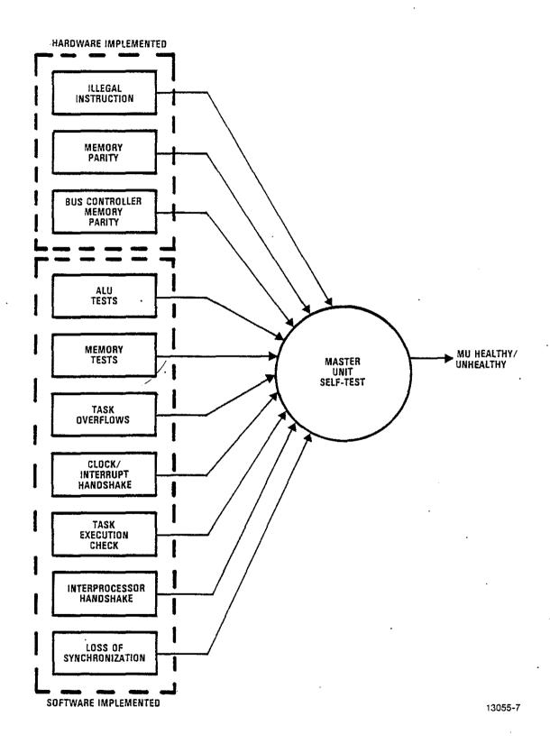
Figure 7. Built-in-Tests for Each Master Unit
