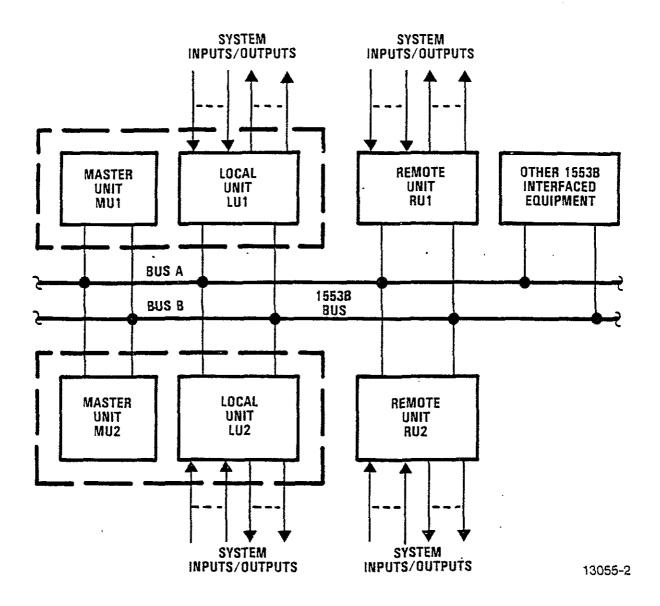
Figure 2. Architecture of the Integrated Multiplex System
