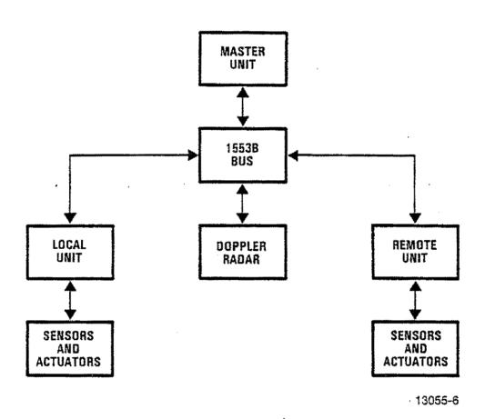
Figure 6. Hierarchy of Elements Covered by BIT/RM
