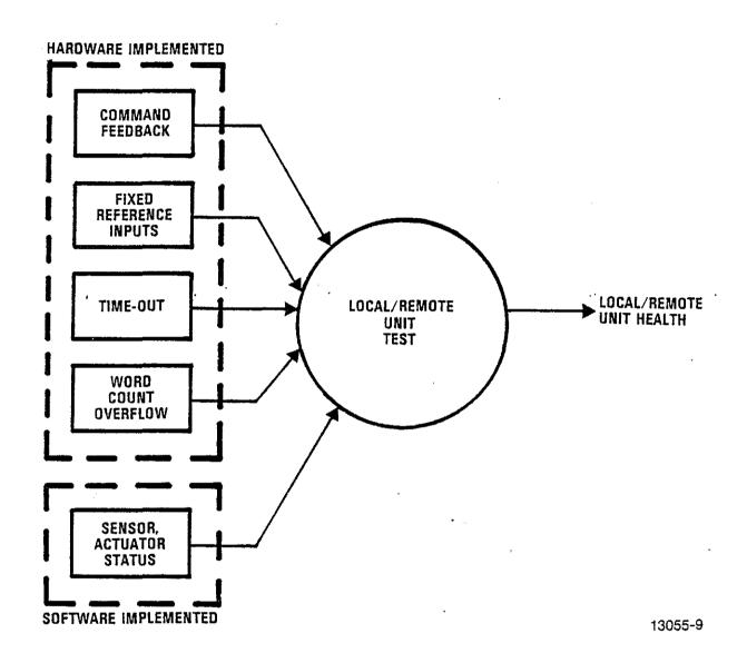
Figure 9. Built-in-Tests for Each Local and Remote Unit
