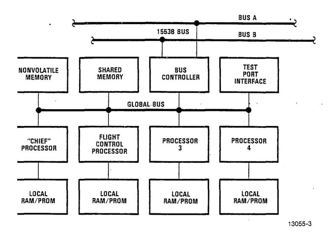
Figure 3. Architecture of Each Master Unit
