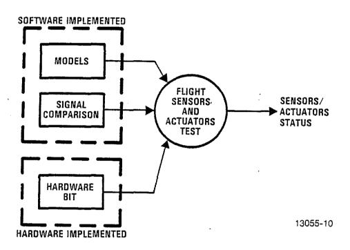
Figure 10. Built-in-Tests for the Flight Control Sensors and Actuators
