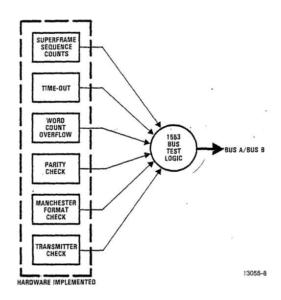
Figure 8. Built-in-Tests for Each 1553 Bus
