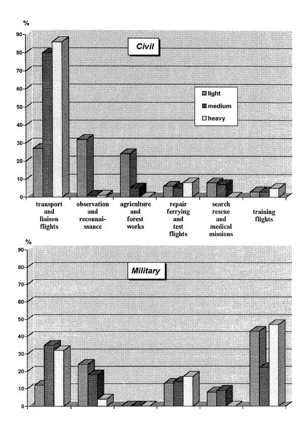
Fig. 1. Flight task distribution of air accidents
