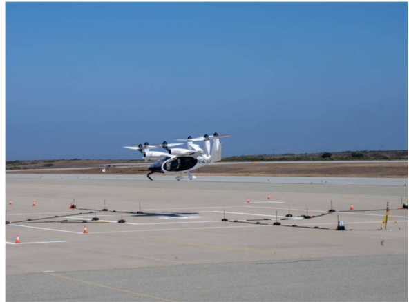
Fig. 21. Real-world characterization of the outwash below an eVTOL aircraft will be prone to significant error, especially if the complexity of the underlying physics is not fully appreciated. (Image from Ref. 5.)
