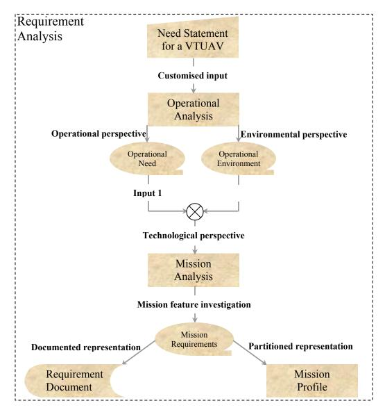
Fig 1.2: Requirement analysis to investigate the required performances and design constraints for a generic VTUAV design
