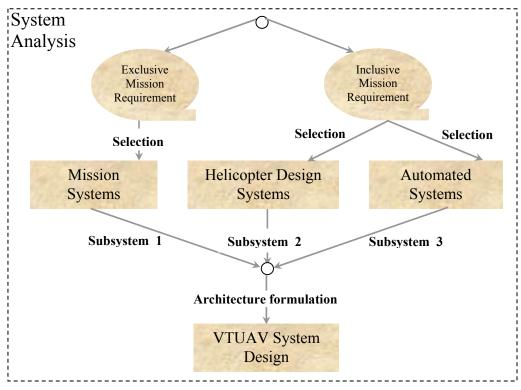
Fig 1.3: System analysis to identify system elements for a generic VTUAV design
