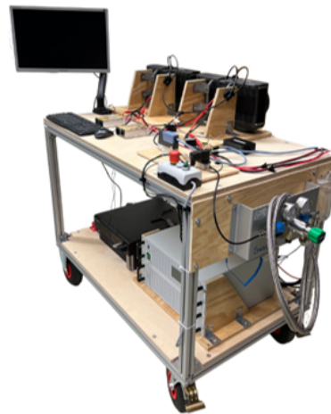
Figure 4: Mobile Hydrogen Fuel Cell and Battery Test-bench with capacity up to 9.6kW and hydrogen pressure regulator
