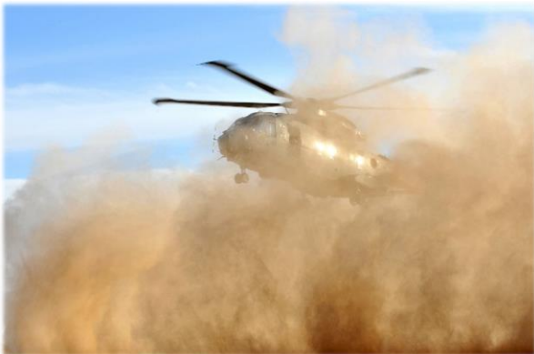
Figure 1: A Royal Air Force AW-101 'Merlin' Helicopter performing a landing manoeuvre in brownout conditions (Courtesy of MoD Defence Imagery).
