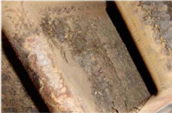
Figure 2: Dust deposition on a nozzle guide vane looking at the leading edge [11].
