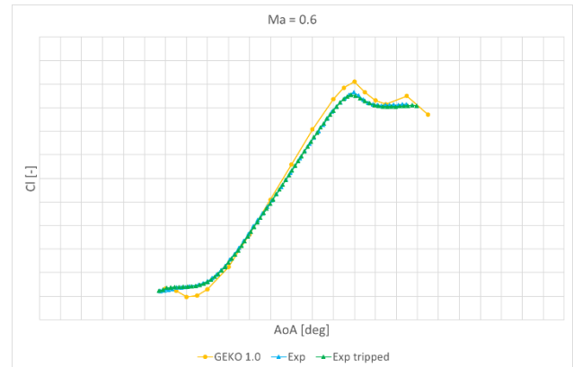
Figure 30: Legacy-12 Lift Coefficient vs Angle of Attack at Mach 0.6
