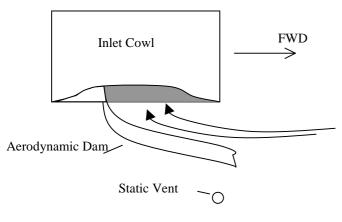
Figure 5. Aerodynamic dam fitted to the original ACS inlet cowl
