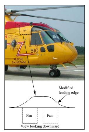
Figure 4. EH101 CSH with the re-shaped ACS inlet cowl
