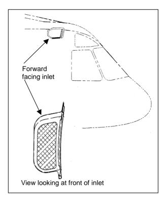
Figure 8. Forward facing ACS Inlet on the EH101 Civil
