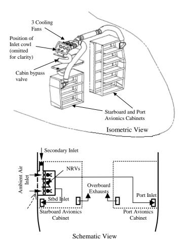
Figure 2. Isometric View and Schematic View of the EH101 Avionics Cooling System
