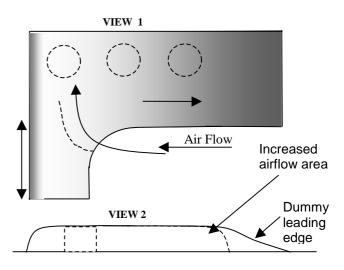
Figure 7. Final/optimal standard of ACS inlet cowl
