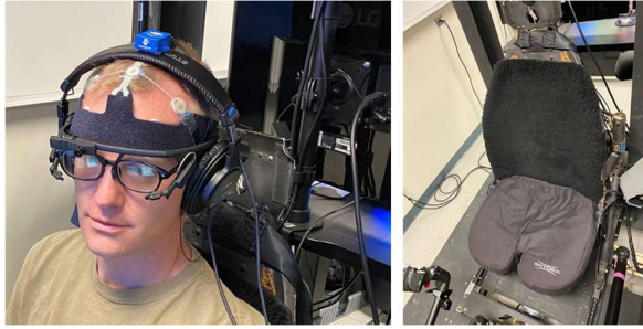
Figure 14: Left: Participant wearing the Sennheiser Game 1 headphones with head-tracker, EEG sensors and Pupil Lab Core eye-tracker. Right: Tactile Seat Bottom Cushion (Engineering Acoustics Inc.)
