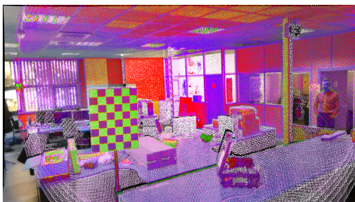
Figure 9: Picture of one of the scenes used for the calibration showing the point cloud projected on the image
