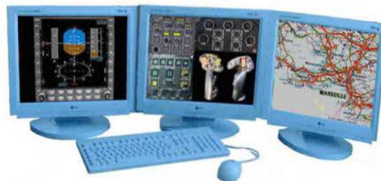
Fig. 12 - Pictorial view of a NH90 PTT
