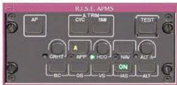
Fig. 10 – EC155 virtual Auto Pilot Panel
