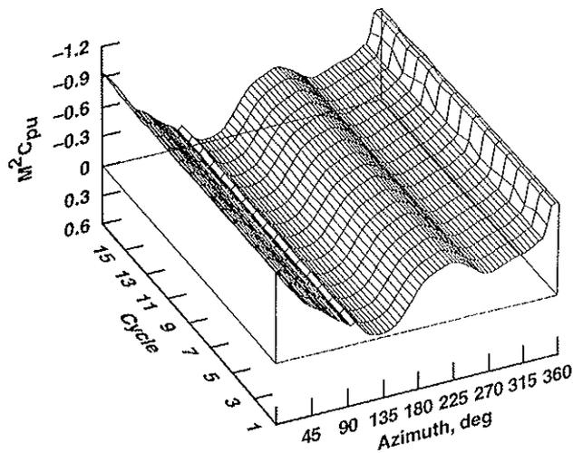
Figure 7. Upper surface pressure as a function of blade azimuth and cycle number (Counter 8534);  $x/c = 0.030$ ,  $r/R = 0.865$ ,  $C_w/\sigma = 0.08$ , advance ratio = 0.368, 0 to 60 harmonics.
