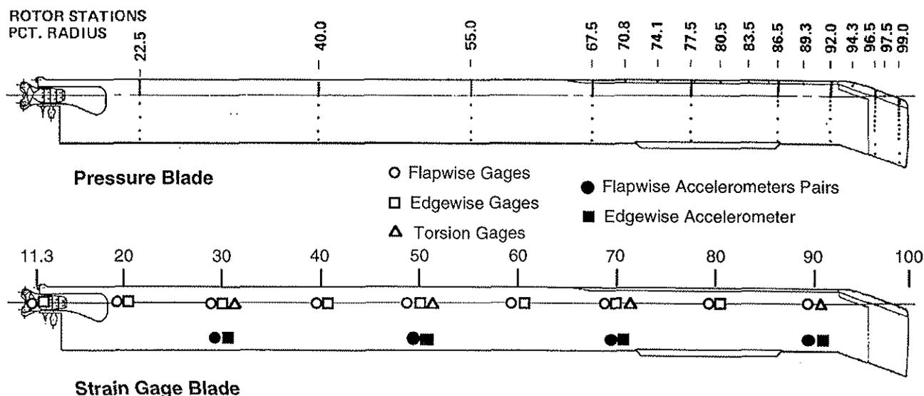
Figure 2. Schematic of pressure transducer, strain-gage and accelerometer locations along UH-60A rotor blades.
