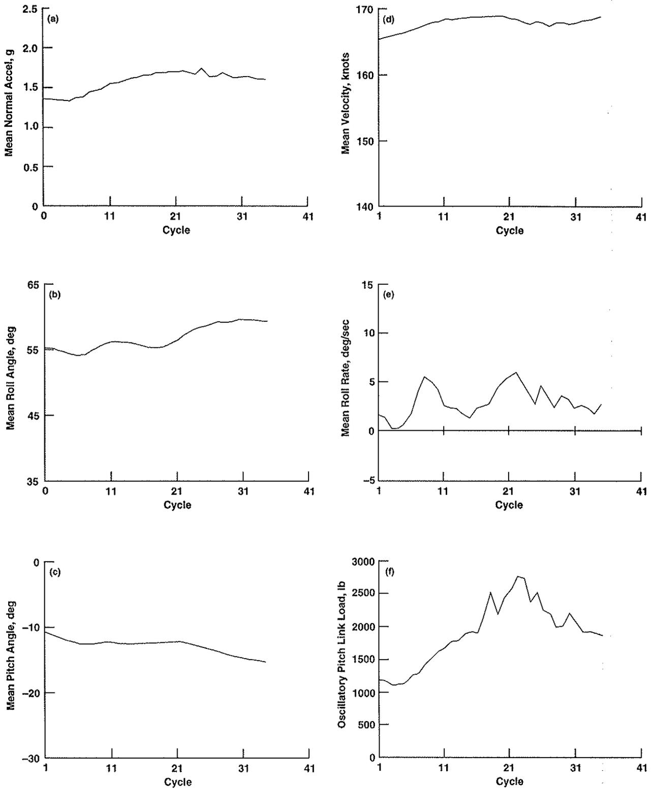
Figure 9. UH-60A a) mean load factor, b) mean roll attitude, c) mean pitch attitude, d) mean airspeed, e) mean roll rate, and f) mean pitch-link load for each rotor cycle of an high speed steady right turn (Counter 11679).
