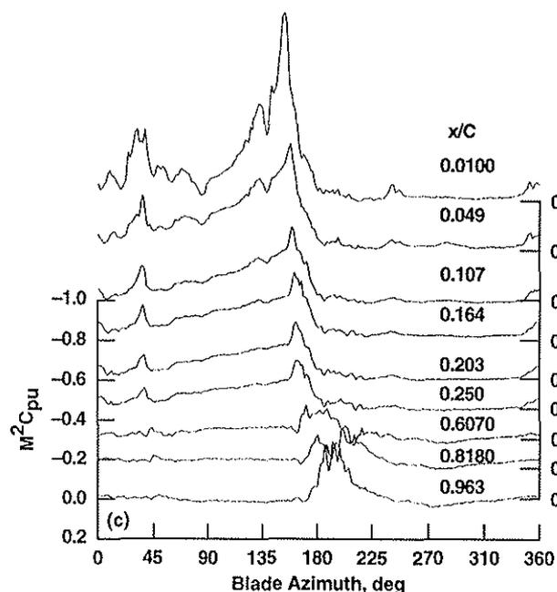
Figure 12. a) Section normal force, b) section moment, and c) an offset plot of upper surface pressures vs rotor azimuth for  $r/R = 0.225$ , (Cycle 22, Counter 11679); 0 to 60 harmonics.
