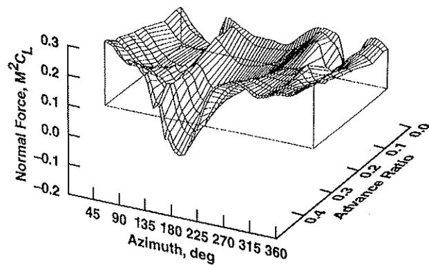
Figure 5. Section normal force as a function of blade azimuth and advance ratio;  $C_w/\sigma = 0.08$ ,  $r/R = 0.92$ , 0 to 60 harmonics.
