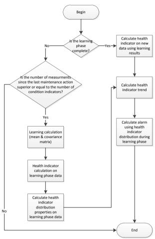
Figure 2: Anomaly detection process
