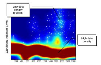
Figure 8 – Outlier detection based on data density function
