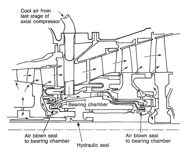
Fig.10 Turbine bearing chamber
