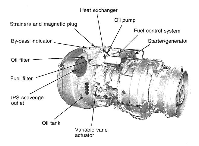
Fig.8 External view of engine
