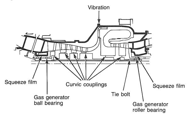
Fig.9 Gas generator shaft arrangement
