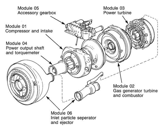
Fig.7 Engine modules
