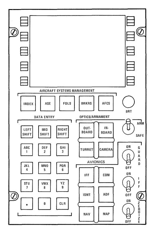
Figure 4: Control and Display Unit
