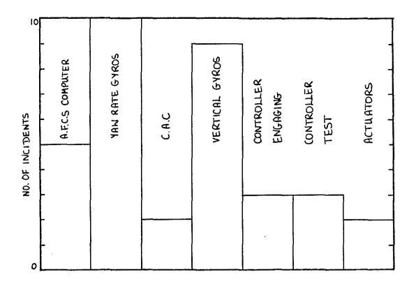
FIG. 44 A.F.C.S. FAILURES - LYNX DEVELOPMENT TRIAL
