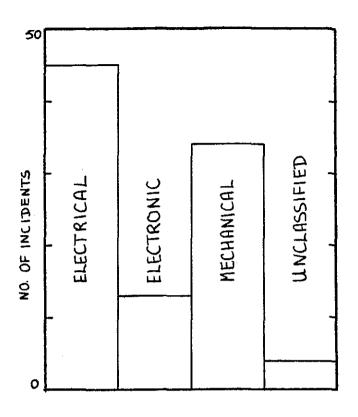
FIG. 9 TYPES OF FAILURE - LYNX DEVELOPMENT TRIAL
