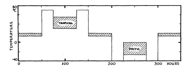
FIG. 2 TEMPERATURE CYCLE - 2ND. WASP TRIAL
