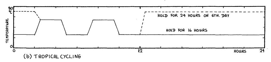
FIG. 3 TEMPERATURE CYCLES - SEA KING TRIAL
