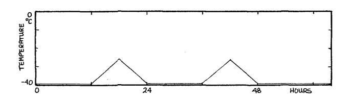
FIG. 8 ENVIRONMENTAL SOAK CONDITIONS - LYNX PRODUCTION TRIAL
