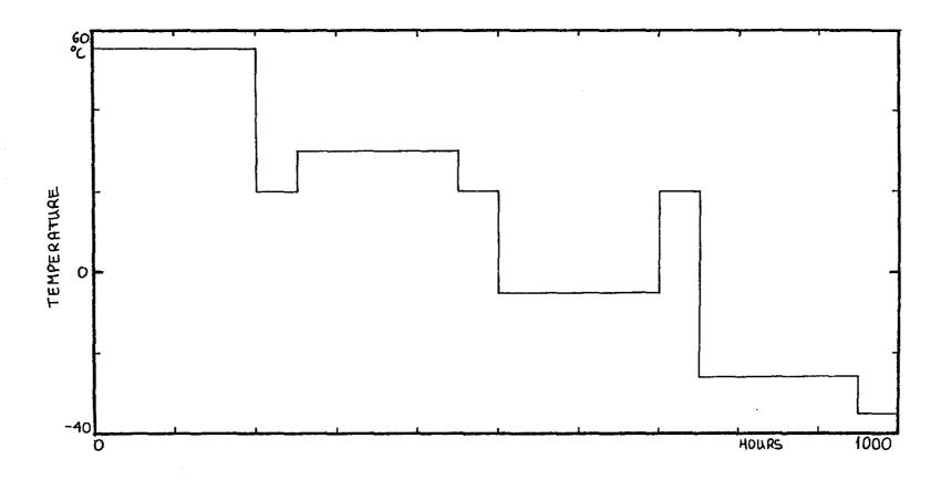
FIG. 7 ENVIRONMENTAL RUNNING CONDITIONS - LYNX PRODUCTION TRIAL
