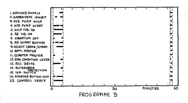
FIG. 5 RIG CONTROL PROGRAMMES - LYNX PRODUCTION TRIAL
