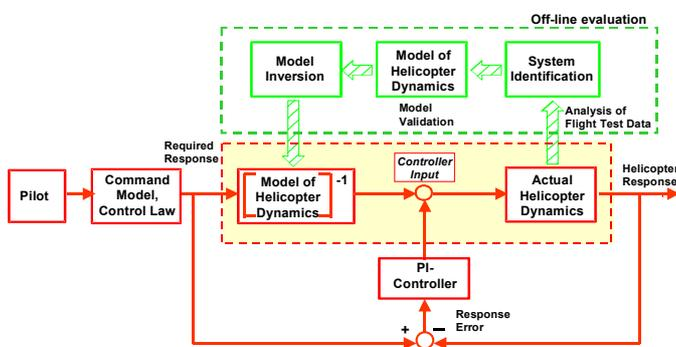
Figure 9: Principle of Model Following Control System (MFCS)
