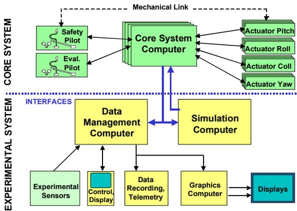
**Figure 2:** FHS system architecture
