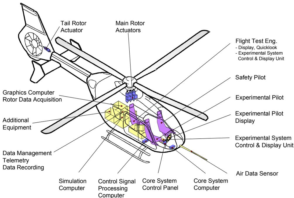
**Figure 3:** FHS modifications and additional equipment
