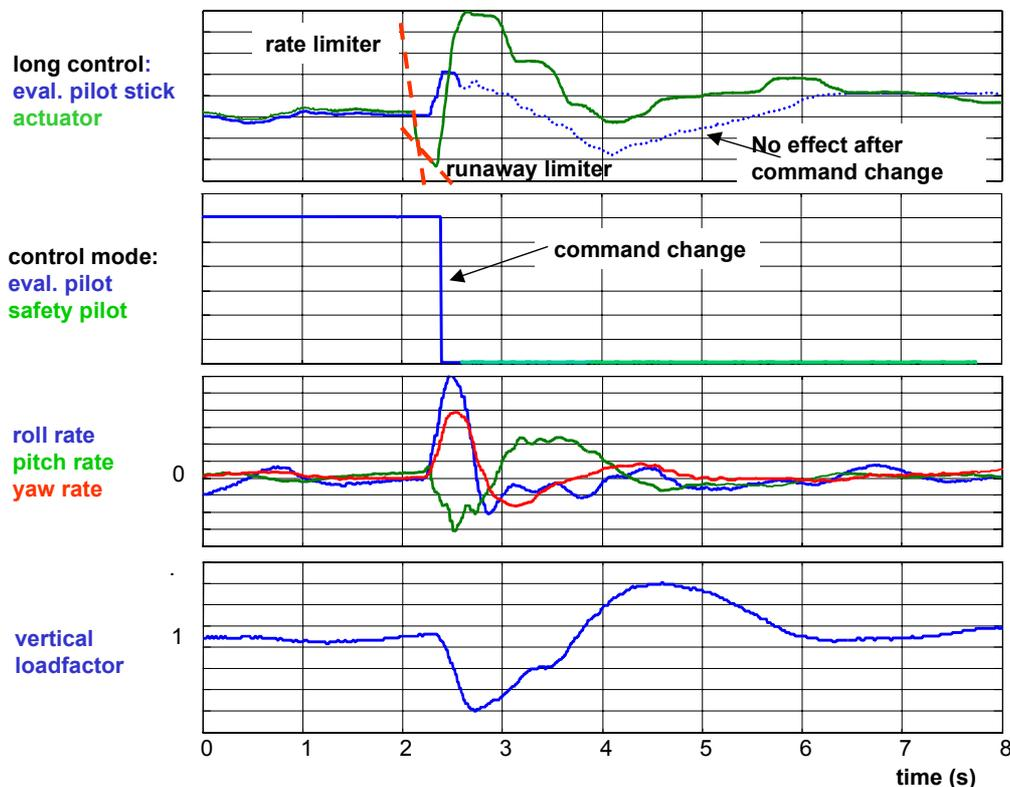
**Figure 5:** Runaway Test: Demonstration of limiter efficiency, mode change and helicopter response
