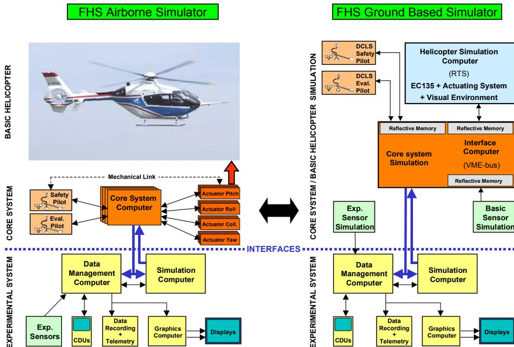
Figure 8: Comparison of the system architectures of the FHS and the FHS ground simulator
