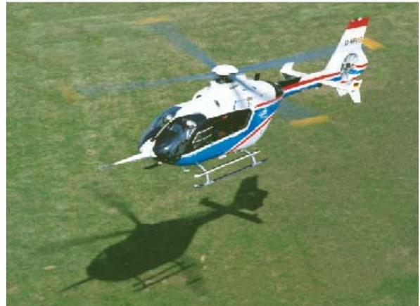
**Figure 1:** The Flying Helicopter Simulator EC135 (FHS)
