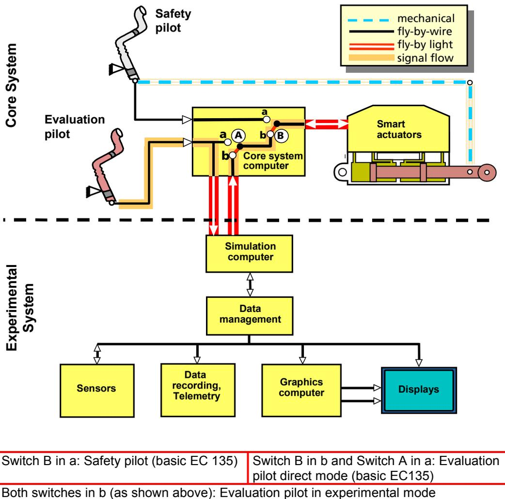
**Figure 4:** Principle of FHS control modes
