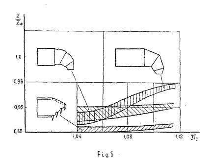
The investigation carried out show that optimization of geometry and flow pattern may help to reach a low level of losses in the gas dynamical path components, and the total power consumption to
