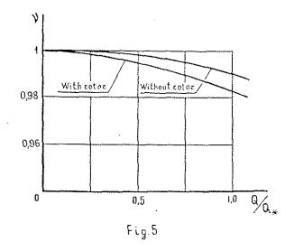
pressure ( $\pi_c \sim 1,1$ ) zone. The nozzle efficiency was evaluated by one jet turn losses as a ratio between measured Z and ideal Z\* forces. If the nozzle is made to turn the flow in only one plane the nozzle losses may be reduced by practically two times as compared that of a more general configuration nozzle (fig. 6).
