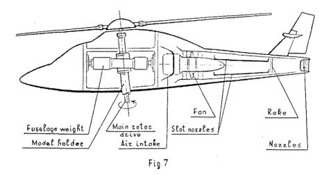
To investigate the behaviour of an air jet nozzle controlled helicopter in the oblique flow conditions a mechanized model was prepared for wind tunnel testing (fig. 7). The air jet nozzle system with two slots ensures the stable circular flow and required helicopter balancing and control margin parameters in a wide range of attack and slip angles, (fig. 8).
