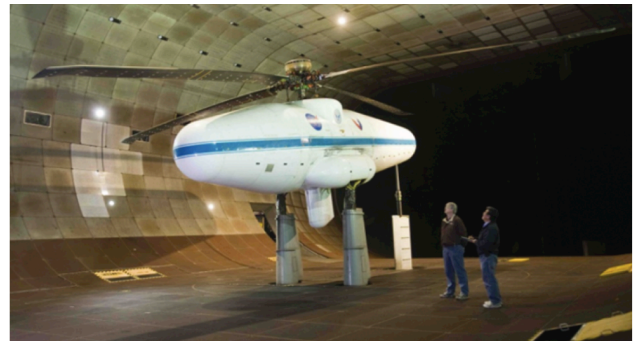
Figure 1 UH-60A rotor system installed on the Large Rotor Test Apparatus (LRTA) in the NFAC 40-by 80-Foot Wind Tunnel
