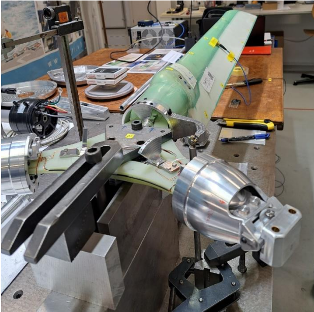
Figure 8: Fixed-free yoke-blade assembly GVT test set-up
