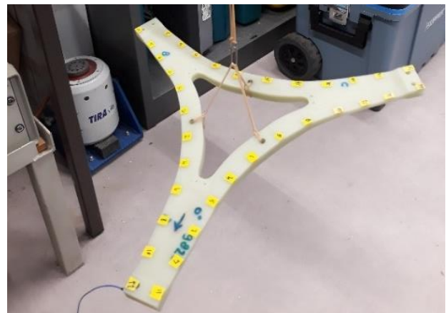
Figure 4: Free-free yoke GVT test set-up
