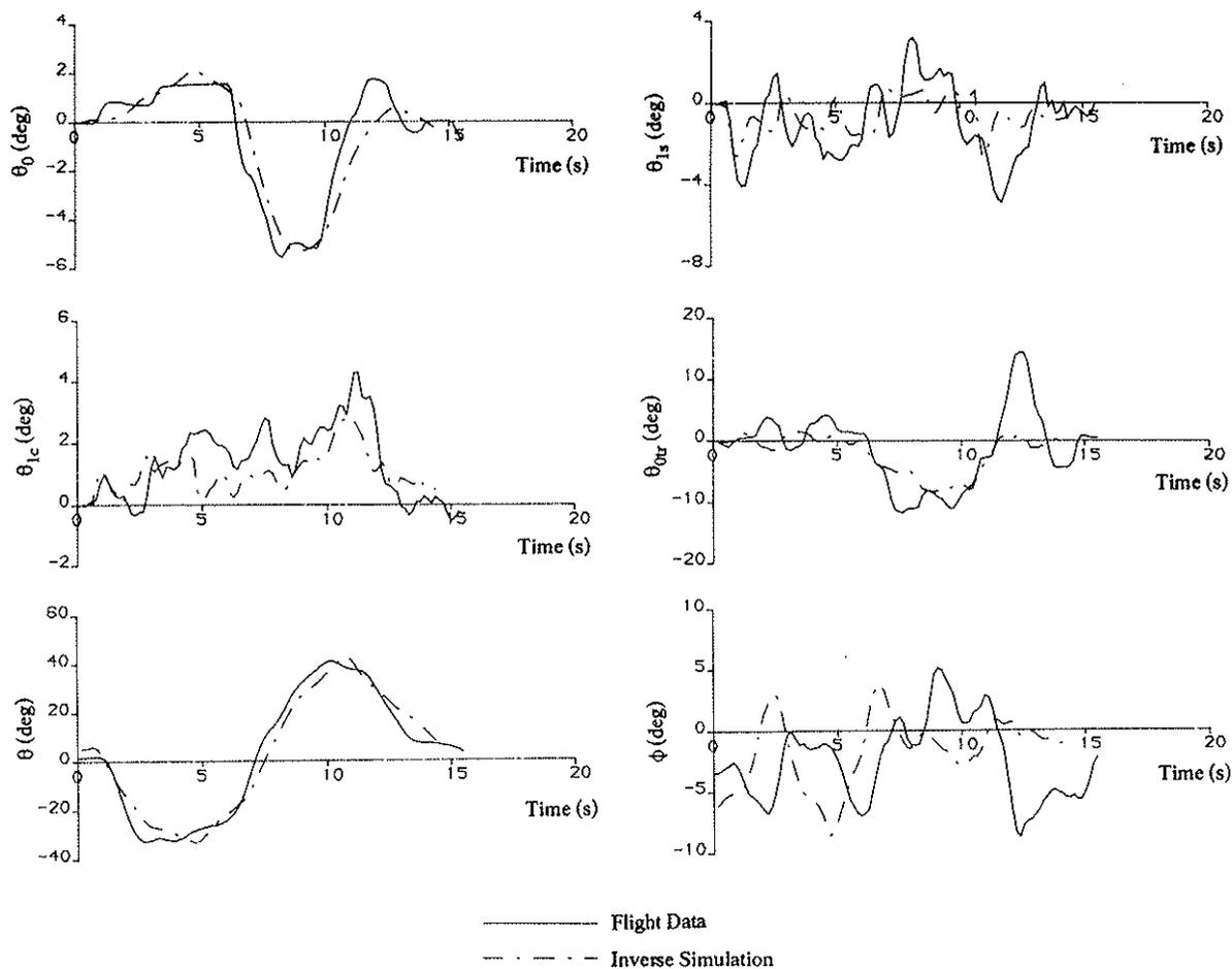
**Figure 2 :** Comparison of Control and Attitude Time Histories for Westland Lynx Helicopter Flying a 600ft Quick-hop Manoeuvre
