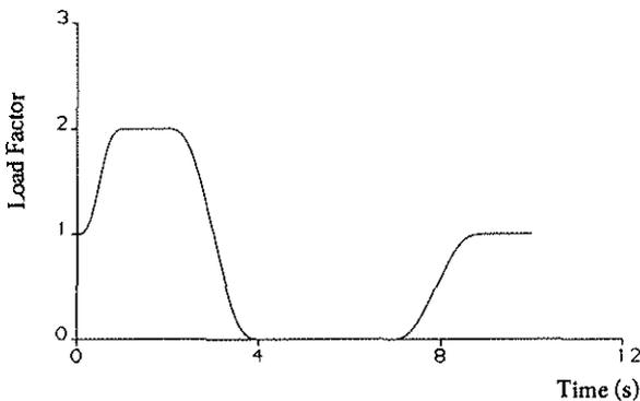
**Figure 9** : Load Factor Distribution in Pull-up/Push-over MTE
