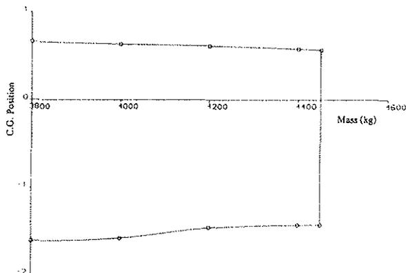
Figure 18 : Centre of Gravity and Mass Envelope for "Configuration 3" Flying Acceleration and Deceleration MTE
