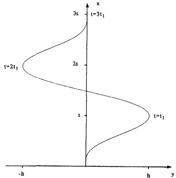
Figure 4 : Track for the Slalom MTE
