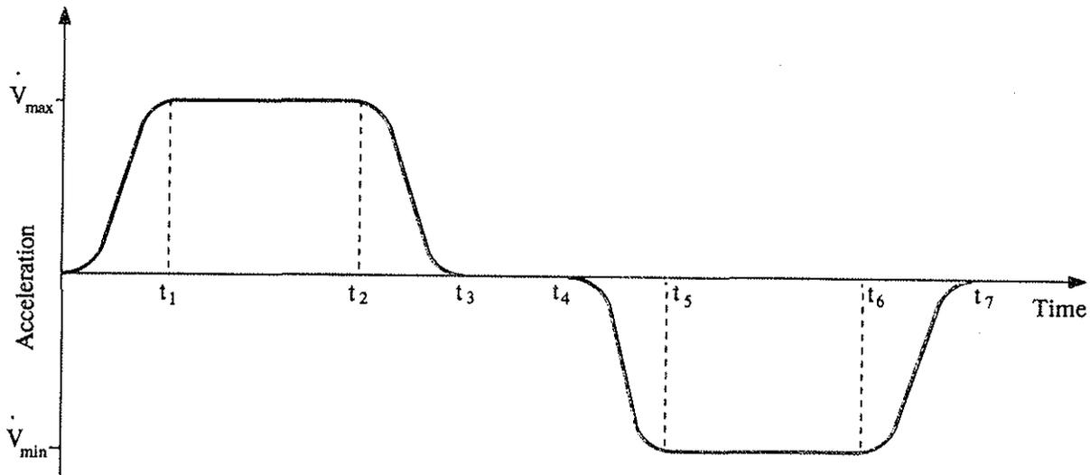
Figure 7 : Acceleration Profile for a Rapid Sidestep MTE
