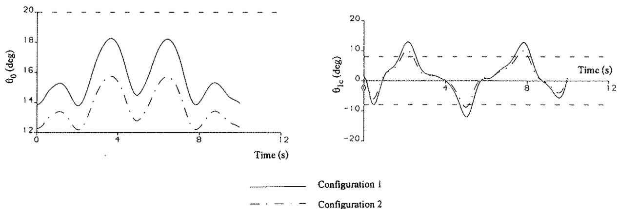
**Figure 13 : Control Inputs Required to Fly a Slalom MTE**
