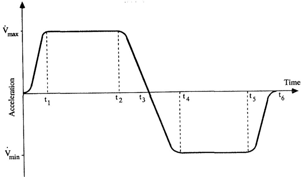
**Figure 5** : Acceleration Profile for an Acceleration and Deceleration MTE
