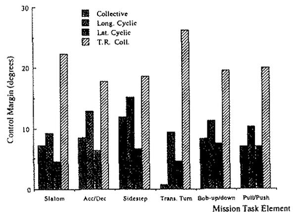
**Figure 17 : Control Margins of "Configuration 3" Flying a Series of MTEs**
