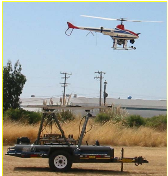
Figure 14 Vision-based Landing of a VTOL UAV on a Simulated Ship Deck
