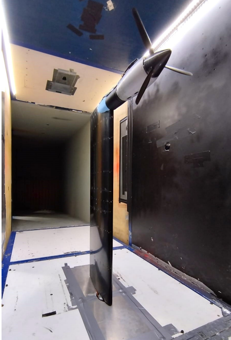
Figure 2: Wing-propeller model mounted inside the wind tunnel test section.
