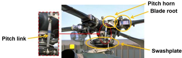
Fig. 1: MBB Bo105 main rotor head and swashplate assembly. Adapted from ©1988 Burkhard Domke<sup>[2]</sup> and used with permission.
