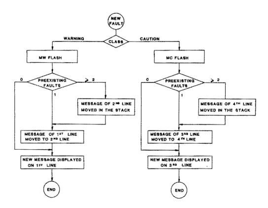
Fig. 4 LOGIC FLUX DIAGRAM
