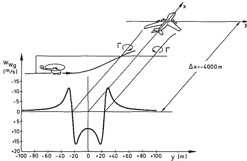
Figure 22: B 747-Trailing-Vortices Penetration during Takeoff
