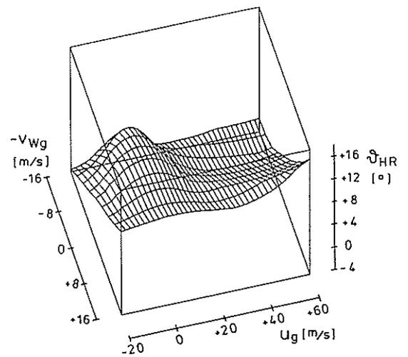
Figure 4: Tail Rotor Collective Blade Angle as Function of Airspeed
