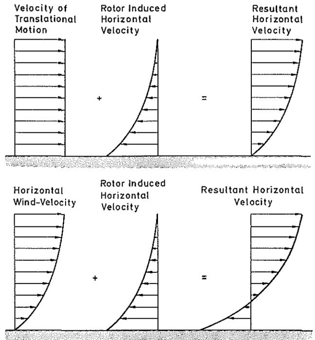
Figure 8: Resultant Horizontal Velocity in Ground Effect in Case of Translational Motion and Wind
