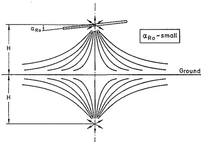
Figure 5: Source Model in Ground Effect
