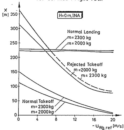
Figure 21: Wind Influence on Takeoff and Landing Distance
