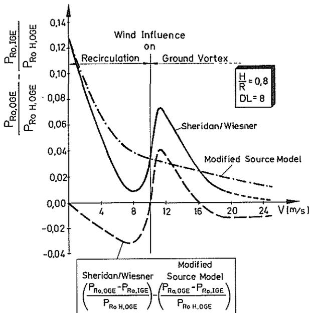
Figure 10: Non-Dimensional Main-Rotor-Power-Required-Difference between OGE- and IGE-Case
