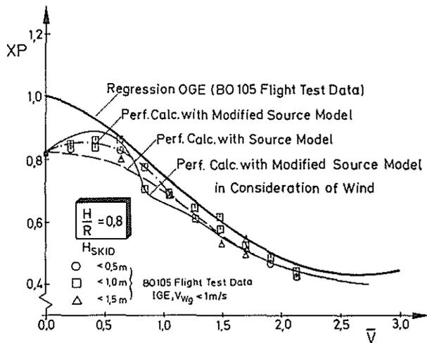
Figure 13: Influence of Ground Effect on Power Factor in Forward Flight
