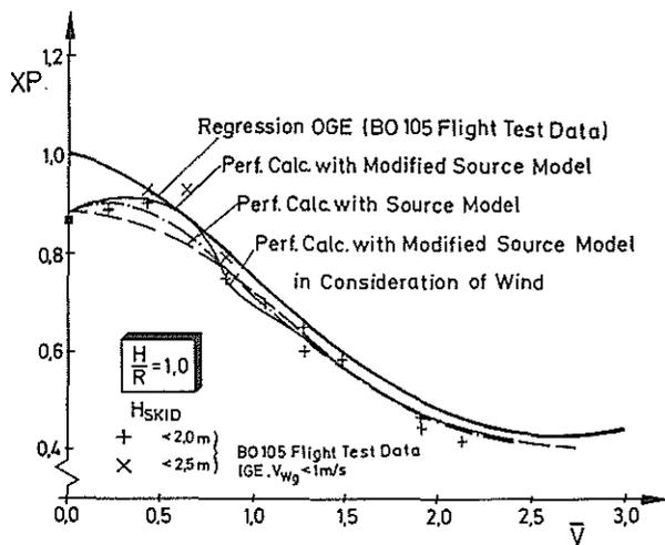
Figure 14: Influence of Ground Effect on Power Factor in Forward Flight
