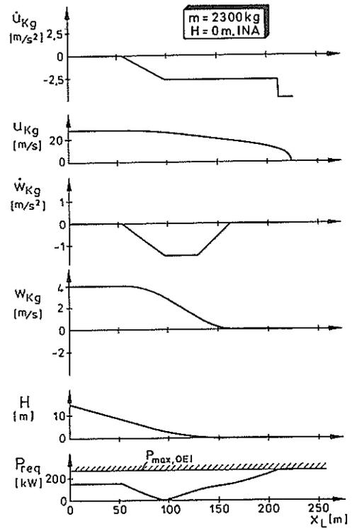
Figure 18: Approach with One Engine Inoperative ( $u_{Wg} = 0$  m/s)
