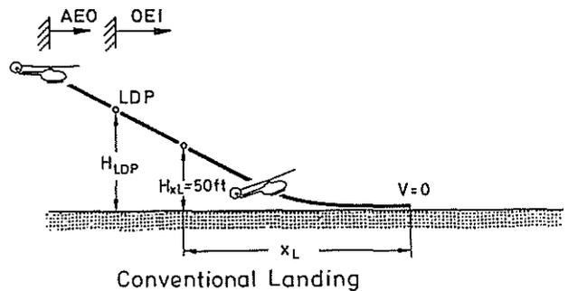
Figure 15: Takeoff- and Landing Profiles
