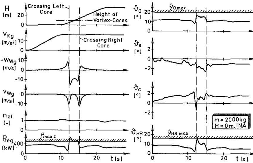
Figure 24: Normal Penetration of Trailing Vortices (  $x=-4000m$ ) during Helicopter Takeoff with Defined Flight Path
