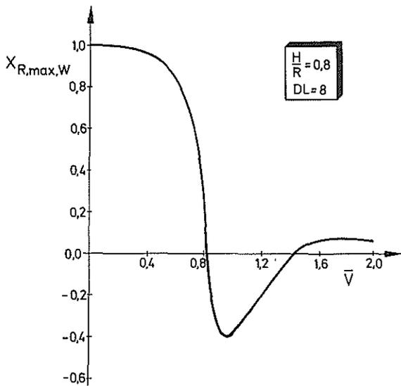
Figure 12: Maximum Recirculation Factor in Case of Wind
