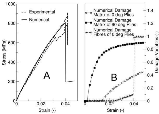
Fig. 23: Numerical-Experimental correlation of the tensile response for ([0][90])ns lay-up (A) and numerical damage variables in the different plies (B).
