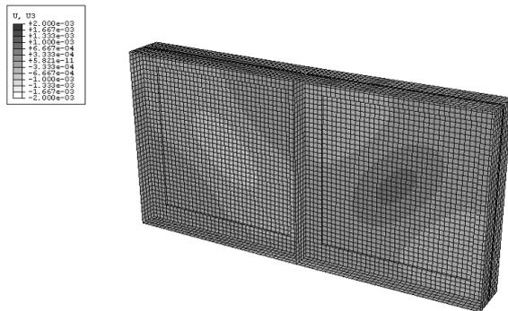
Fig. 9: Out-of-plane deformation at 37 kN.
