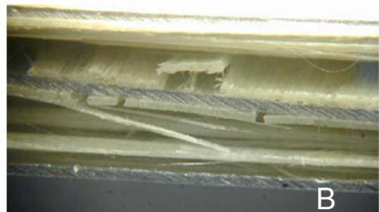
Fig. 25: Evolution of the damage variables obtained with the material model developed for the composite plies (A) and experimental damage observed in a failed Glare specimen (B).
