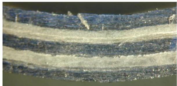
Fig. 3: Section of a Glare 3-3/2 after a low energy impact test
