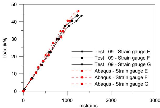
Fig. 13: Strains of the stretched diagonal.
