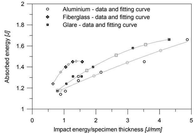
Fig. 2: Absorbed energy levels vs. impact energy in low energy impact tests.
