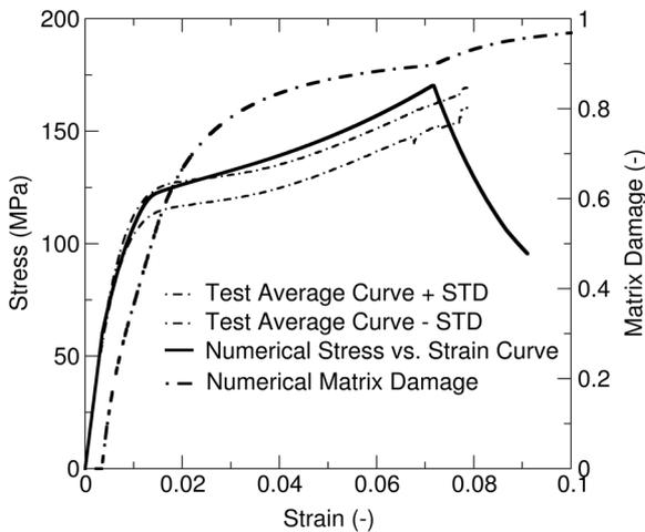
Fig. 21: Numerical-experimental correlation and numerical damage of the  $([+45] [-45])_{ns}$  lay-up response.
