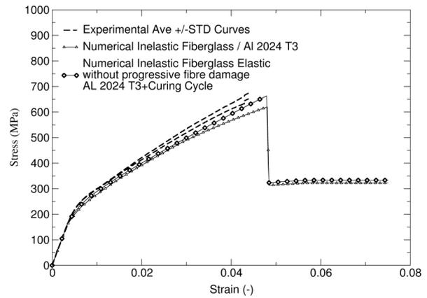
Fig. 24: Numerical-Experimental correlation of the full-range (A) response of Glare 3-3/2 obtained with inelastic composite layers.
