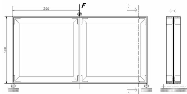
Fig. 6: Wagner's web configuration used for the numerical-experimental correlation.
