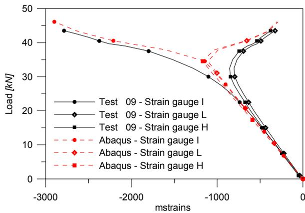
Fig. 12: Strains on the compressed diagonal.
