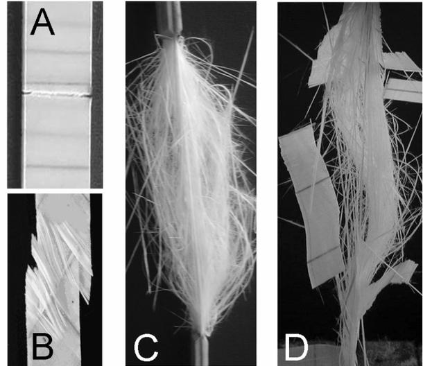
Fig. 17: Failure modes of different fiberglass laminates.
