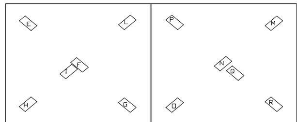
Fig. 11: Locations of the strain gauges on Glare panels.
