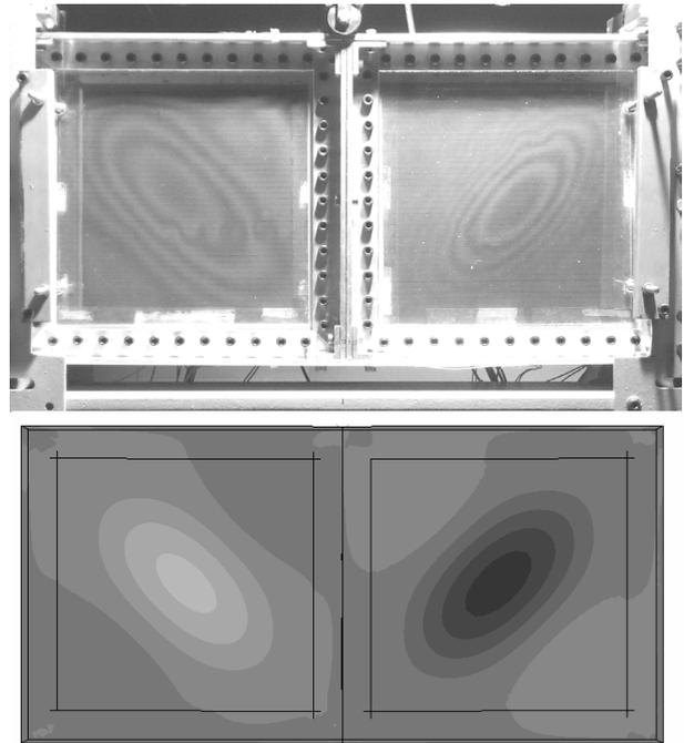
Fig. 14: Out-of-plane deformation at 37.5 kN.
