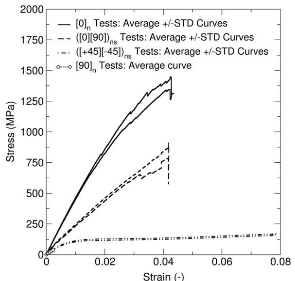
Fig. 18: Stress-strain curves of different fiberglass laminates.
