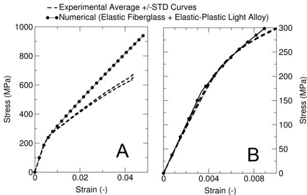
Fig. 16: Numerical-experimental correlation of the Glare 3 3/2 tensile behaviour using an elastic fiberglass model.
