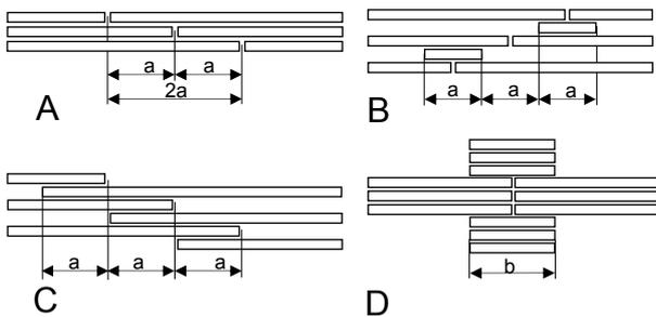
Fig. 4: Different joint configurations tested in the experimental activities.
