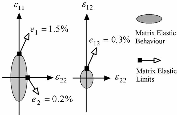
Fig. 20: Calibration of the limits of the elastic behaviour for the matrix phase.
