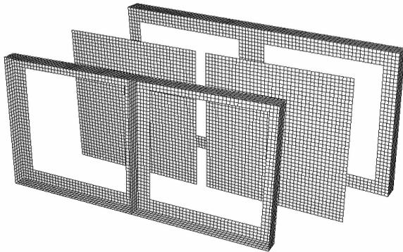
Fig. 7: Finite element model of the Wagner's web: frontal and rear frames, Glare flat panels.
