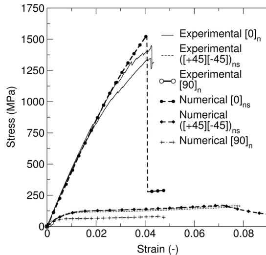
Fig. 22: Verification of the calibrated material model with the numerical-experimental correlation for the  $[0]_n$ ,  $[90]_n$ ,  $([+45] [-45])_{ns}$  tests.
