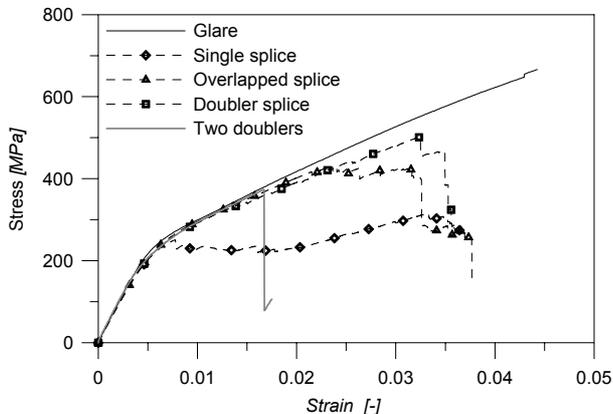
Fig. 5: Tensile response of differently joined Glare panels.
