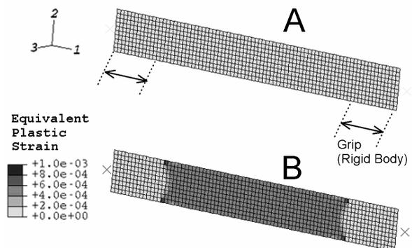
Fig. 15: Model of the Glare 3-3/2 tensile specimen (A) and analysis (B).
