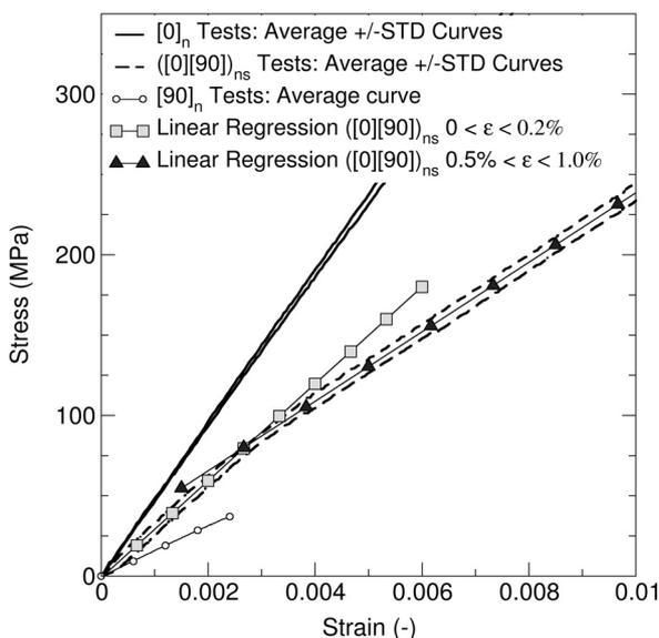
Fig. 19: Bi-linear response of  $([0][90])_{ns}$  fiberglass laminates.
