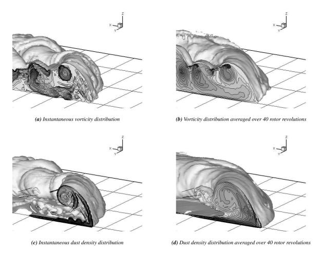
Figure 3: Vorticity and dust distributions in the flow below a tandem rotor helicopter during a landing manoeuvre – normalised advance ratio  $\mu^* = 0.29$  ( $\mu = 0.025$ ). Darker contours represent higher values of the variable within each plot.
