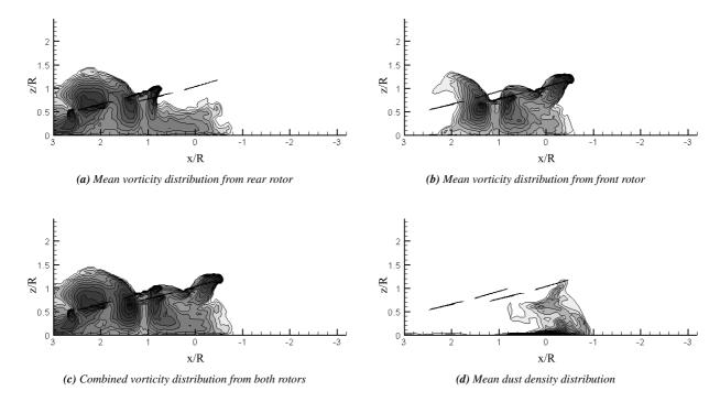
Figure 4: Vorticity and dust distributions in the flow below a tandem rotor helicopter during a landing manoeuvre – normalised advance ratio  $\mu^* = 0.47$  ( $\mu = 0.04$ ). Darker contours represent higher values of the variable within each plot.
