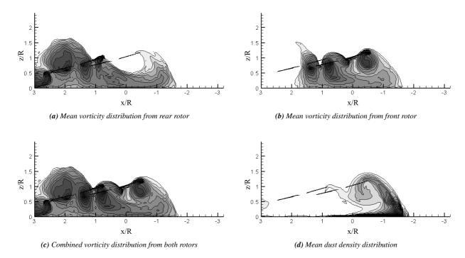
Figure 5: Vorticity and dust distributions in the flow below a tandem rotor helicopter during a landing manoeuvre – normalised advance ratio  $\mu^* = 0.29$  ( $\mu = 0.025$ ). Darker contours represent higher values of the variable within each plot.
