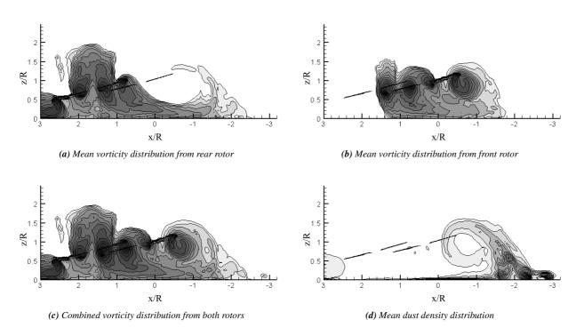
Figure 6: Vorticity and dust distributions in the flow below a tandem rotor helicopter during a landing manoeuvre – normalised advance ratio  $\mu^* = 0.12$  ( $\mu = 0.01$ ). Darker contours represent higher values of the variable within each plot.
